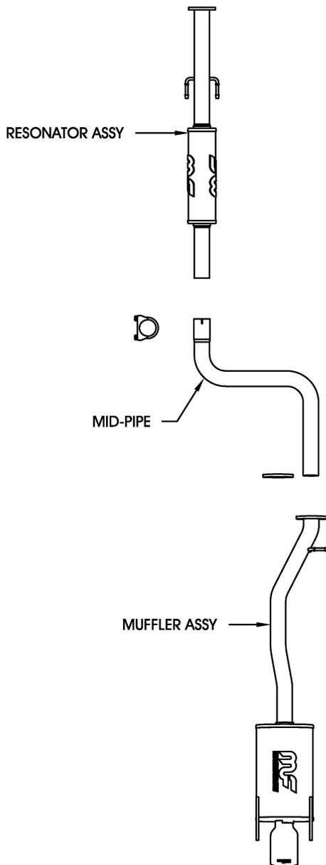
**Step 1:** (Carefully read all instructions before installation) Unbolt the OEM muffler from the extension pipe in front of the rear control arm. Remove the muffler from the OEM rubber insulators. Do not damage the OEM rubber insulators, as they will be re-used to mount the new system. Unbolt the resonator assembly from the catalytic converter. Do not discard the OEM fasteners, as they may be re-used to mount the new system.
