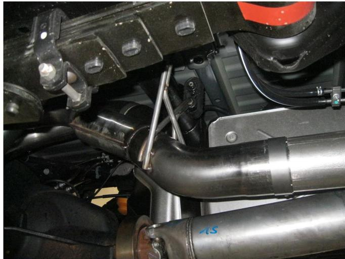
**Step 2.** Begin installation of the Magnaflow system by first clamping the Y-Pipe Assembly inlet to the newly cut outlet of the DPF using the supplied 4.00" clamp. Then attached the two Extension Pipes to the Y-Pipe Assy using the supplied 3.50" clamps and fitting the hangers in the rubber insulators (leave all clamps loose for final adjustment of the complete system). If your vehicle has an O2 sensor re-install at this time. If not, install the provided sensor boss plug.
