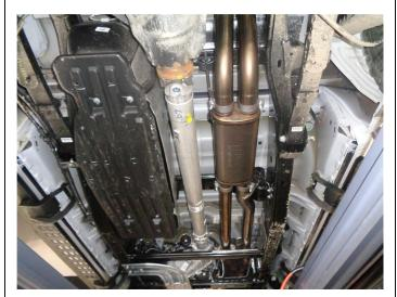
**Step 6.** Install the Muffler Assembly by attaching the inlet nipples to the outlets of both Inlet Pipe Assemblies(SuperCab) or Extension Pipes (SuperCrew). Loosely secure using the supplied clamps. Engage the welded hanger to the rubber insulator.
