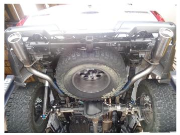
**Step 8.** Finish by loosely attaching both Tail Pipe Assemblies to the Over Axles Pipes using the supplied clamps. Engage the welded hangers to the rubber insulators.
