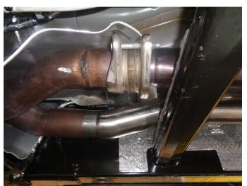
Step 4. - NOTICE - this exhaust kit works with both the SuperCrew and SuperCab models. The SuperCrew has additional parts. Begin the installation by slipping the inlet of the P/S Inlet Pipe Assembly into the OEM band clamp. On the SuperCab model engage the welded hanger into the rubber insulator. Next bolt the D/S Inlet Pipe assembly to the OEM flange junction using the supplied nuts. All clamps and fasteners are to remain loose until final installation.
