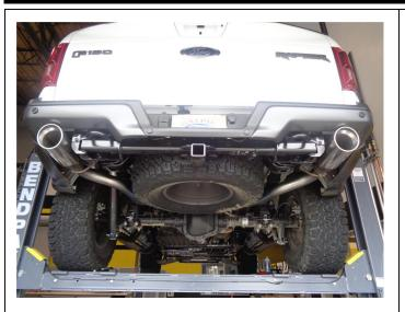
**Step 9.** Once a final position has been chosen for the new exhaust system, evenly tighten all clamps from front to rear using the torque specifications on page one of the instructions. Inspect all fasteners after 25-50 miles of operation and re-tighten if necessary.
