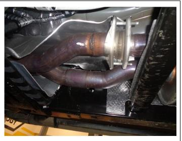
**Step 3.** Finally remove the OEM inlet muffler assembly by unbolting the inlet at the driver side flange junction and loosening the band clamp on the passenger side inlet pipe. Remove the inlet muffler asembly. You are now ready to install your new MAGNAFLOW exhaust system.
