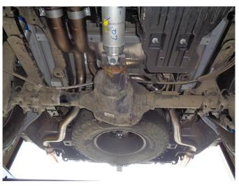
**Step 7.** Loosely attach both Over Axle Pipes to the Muffler Assembly outlets using the supplied clamps.
