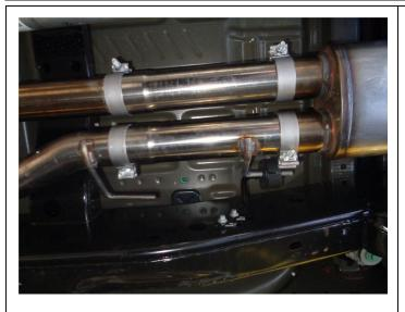
**Step 5.** FOR THE SUPERCREW ONLY, install both extension pipes into the resonator outlets and engage the hanger into the rubber insulator.
