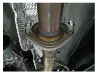
**Step 1:** To remove the OE exhaust system, unfasten the hardware at the inlet flange (Retain fasteners to be re-used).
