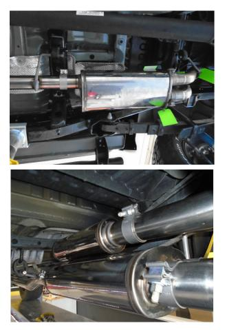
**Step 5:** Next attach the Oval Muffler to the Inlet Pipe with the supplied 2.50" clamp. This exhaust system is configured to allow the user to tune the sound. For a more moderate exhaust sound install the U-pipe Assy and the 4.00" NDT Chamber (as shown) using the suppled 2.50" clamps. For a more aggressive sound see configuration chart below.
