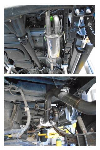
**Step 6:** Attach the Over Axle Pipe to the Muffler Assembly as shown using the provided 2.50" clamp and the OE rubber insulator.
