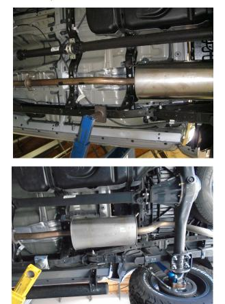
**Step 2:** Working front to rear, disengage all welded hangers from the rubber insulators and remove the system. (Retain the rubber insulators as they will be needed to mount the new MagnaFlow system.)
