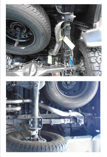
**Step 7:** Before installing the Tailpipe Assembly loosely fit the appropriate Hanger Clamp Assembly from the rear of the tailpipe. Hanger Assemblies are divided by year spread, 2005-2011 and 2012 -2015. Once fitted, install the Tail Pipe Assembly to the Over Axle Assembly using the supplied 2.50" clamp and fit the Hanger Assembly into the rubber insulator.
