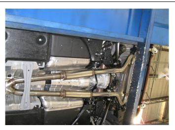
**Step 4.** Loosely secure the Muffler Assembly and both Tip Assemblies in a similar fashion and reattach the cross brace.
