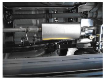
**Step 1.** To remove the OEM exhaust system, you will need to loosen the clamp behind the OEM muffler. Disengage the welded hangers from the rubber insulators. Remove the OEM exhaust system. Do not damage or discard the OEM fasteners or rubber insulators as they will be resued to mount your new MAGNAFLOW system.
