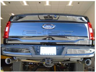
**Step 8.** Once a final position have been choden for the new exhaust system, evenly tighten all clamps from front to rear using the torque specifications on page one of these instructions. Inspect all fasteners after 25-50 miles if operation and re-tighten if necessary.
