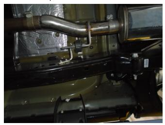
**Step 2. Install your** new MAGNAFLOW system by loosely attaching the Inlet Pipe Assembly using the OE clamp.
