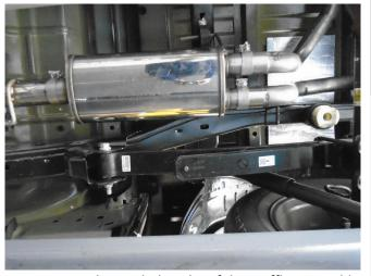
**Step 3.** Loosely attach the inlet of the Muffler Assembly to the outlet of the Inlet Pipe Assembly using the supplied 3.00" clamp. Engage the welded hanger to the rubber insulator.
