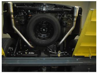
**Step 7. Loosely** Install both Tail Pipe Assemblies using the supplied 2.50" clamps. Engage the welded hangers to the Hanger Bracket Assemblies using the supplied rubber insulators.
