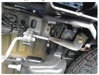
**Step 6.** Attach both Hanger Bracket Assemblies to the vehicles subframe using the supplied hardware as shown.
