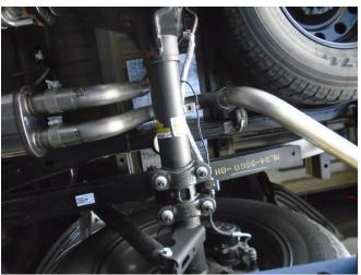
**Step 4.** Loosely attach both Over Axle Pipes to the Muffler Assembly using the supplied 2.50" clamps.
