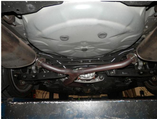
**Step 2.** Next, remove both muffer assemblies by unbolting them from OEM Y-Pipe assembly. Remove all welded hangers from the rubber insulators. The exhaust system may now be removed. Retain all mounting hardware as it will be needed to install your new MAGNAFLOW system.
