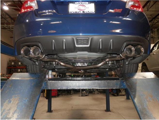
**Step 6.** Once a final position has been chosen for the new system, evenly tighten all clamps from front to rear using the torque specifications on page one of the instructions. Inspect all fasteners after 25-50 miles of operation and re-tighten if necessary.
