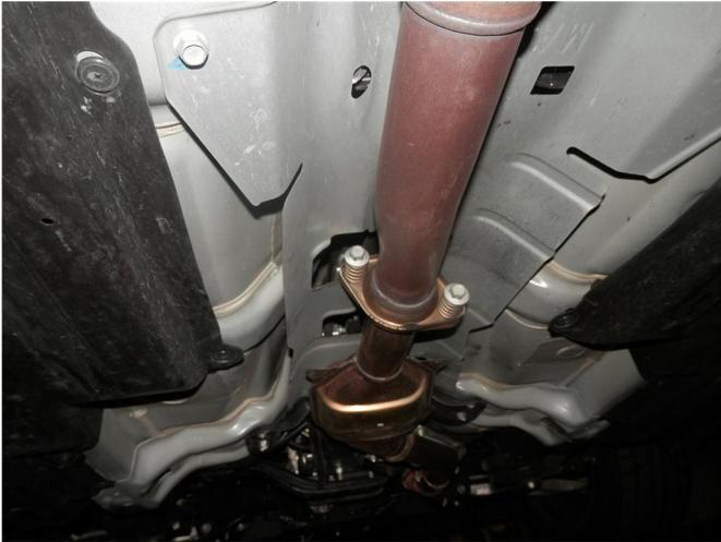
**Step 1.** To remove the OEM exhaust system unbolt the inlet pipe at the catalytic converter flange junction.
