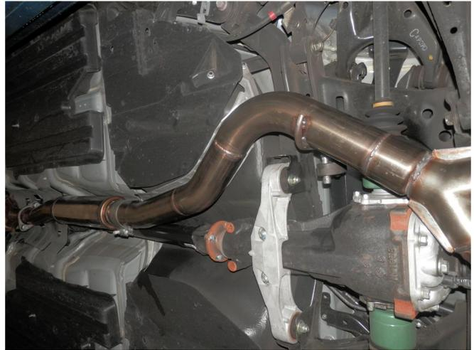
**Step 4.** Next loosely fasten the Y-Pipe Assembly to the Resonator Assembly using the supplied 3.00" clamp. Insert the welded hanger into the OEM rubber insulator.
