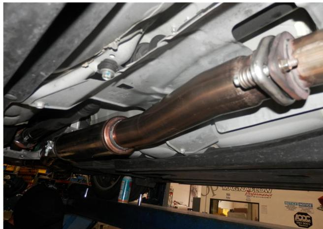
**Step 3.** Begin installation of the new system by fastening the Inlet Pipe Assembly to the outlet of the catalytic converter using the OEM hardware.
