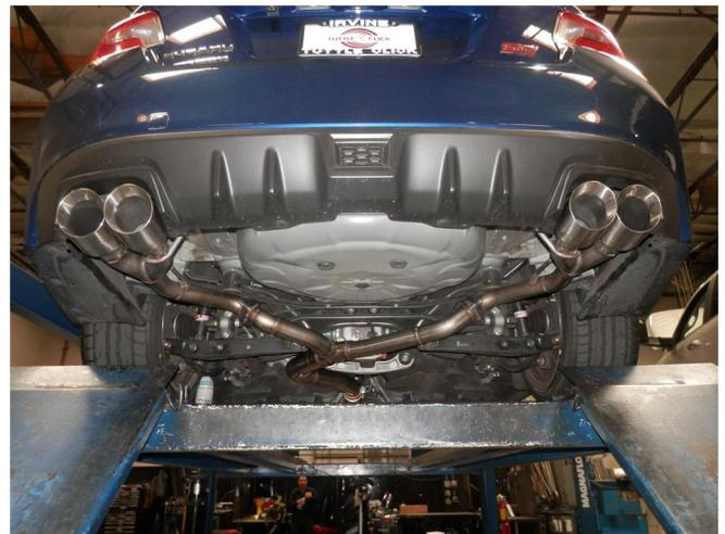
**Step 5.** Next loosely install both Tail Pipes by bolting the inlets flanges to the Y-Pipe Assembly using the OEM hardware. Insert all welded hangers into the OEM rubber insulators.
