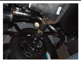
**Step 4.** Install the Over Axle Pipe using the supplied 3.00" clamp. Locate the welded hanger to the OEM rubber insulator.
