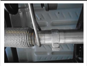
**Step 1.** To remove the OEM exhaust system, loosen the clamp attaching the systems inlet pipe to the catalytic converter outlet pipe. Disengage all welded hangers from the OEM rubber insulators. Do not discard the OEM fasteners or damage the rubber insulators as they will be needed to mount your new MAGNAFLOW system.
