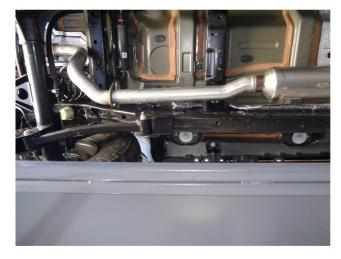
**Step 2:** With the system supported, working front to rear disengage the hangers from rubber insulators and remove the OEM system. Do not discard or damage the clamp or rubber insulators as they will be used to install the new system.
