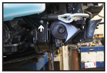
16. Reinstall the washer reservoir using the bracket on the baseplate and new hardware. Reinstall the horn to the lower existing hole (white).
