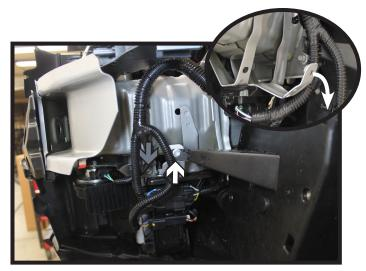
7. On the driver side, using an 8MM socket, remove the screw from the wheel well brace (white). Once the screw is removed, bend the webbing downward far enough for baseplate clearance (inset).
