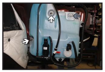
Using a 11MM socket, remove the two (2) nuts from the washer reservoir (white). Then using a 8MM socket, remove the screw (gray). Disconnect/plug all lines and set the reservoir aside.
