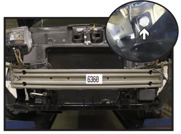
13. Install the baseplate onto the frame and clamp in place. Install the 3/4" bolt and lock washer into the existing hole on the under side of the frame (inset). Insert the 3/4" nut plate on the inside of the frame, level the baseplate and loosely tighten the bolt. Do this on both sides of the vehicle.
