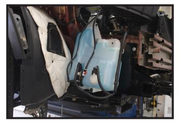
17. Install nine (9) 1/4" washers onto the two (2) studs for the washers reservoir (top). Reinstall the washer reservoir onto the studs and reinstall the factory nuts. The factory screw will not be reinstalled.
