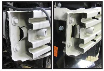
12. Using a reciprocating saw, cut frame and then bend back piece as shown to increase frame access hole. Do this on both sides of the vehicle.
