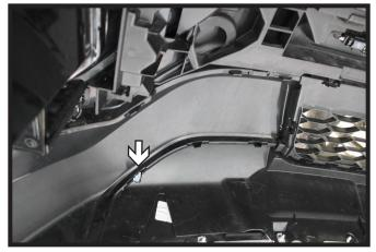
On the backside of the fascia trim the outer tab shown flush with the backside of the fascia for clearance of the baseplate. Do this on both sides of the vehicle.
