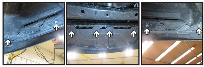
5. Using a T15 Torx, remove the eight (8) bolts from the underside of the fascia. There are two (2) on each side and four (4) in the middle.
