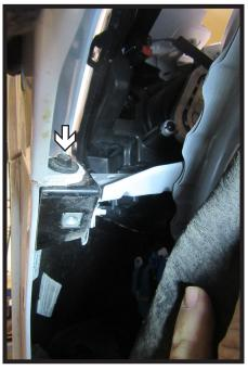
Pull back the wheel well liner. Using a 7MM socket, remove the one (1) bolt at the fascia joint. Do this on both sides of the vehicle.
