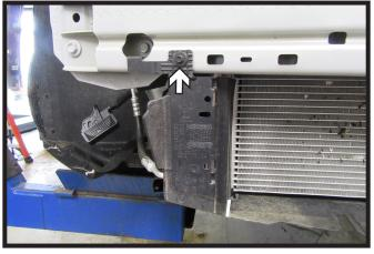
Using a 7MM socket, remove the two
