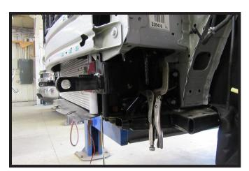
12. Slide baseplate into place. Use large vise grips to hold in place. Do this on both sides of the vehicle.
