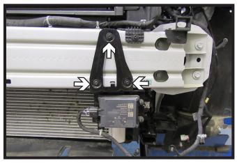
10. Using a 7MM socket, remove the three (3) bolts from the ACC bracket on the driver side of the vehicle. Remove bracket and set aside to be reinstalled later.
