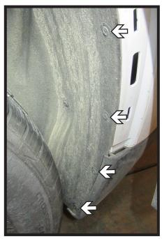
3. Using a T15 Torx, remove the four (4) bolts from the wheel well behind the rear tire. Do this on both sides of the vehicle.
