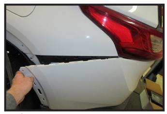
4. Grab the rear panel behind the tire and pull away from the vehicle all the way under the tail light. Do not fully remove panel. Remove tail light and install tail light wiring kit. Once installation is complete, reinstall all items. Do this on both sides of the vehicle.
