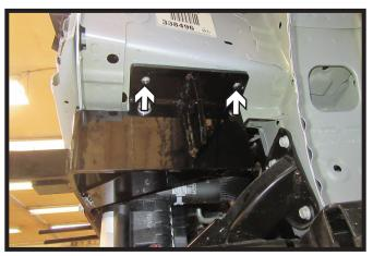
15. Using a 3/8" drill bit, drill the top two (2) holes. Install 3/8" hardware. Do this on both sides of the vehicle.
