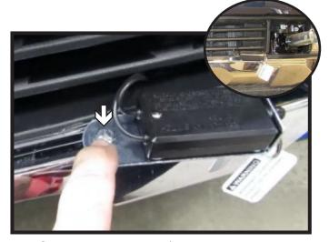
21. Optional: Using a 1/4" drill bit, drill one (1) hole on the driver side of the vehicle. Attach breakaway switch using one (1) 1/4" bolt with hardware.
