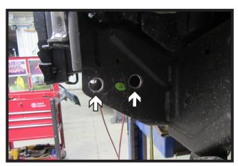
13. Using a 13/16" drill bit, drill out the two (2) tow hook holes. Do this on both sides of the vehicle.
