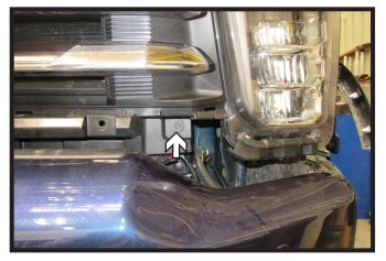
7. Using a 10MM socket, remove the one (1) bolt from the bottom corner of the grill. Do this on both sides of the vehicle.
