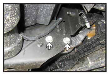
Using an 18MM socket, remove the two (2) bolts from the tow hook. Do this on both sides of the vehicle. Remove tow hooks, they will not be reinstalled.
