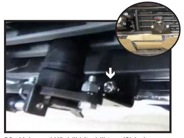
20. Using a 1/4" drill bit, drill two (2) holes on the passenger side of the vehicle using the electrical bracket as a guide. Insert two (2) 1/4" bolts with hardware.
