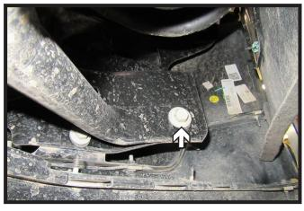
10. Using a 15MM socket, remove the one(1) bolt from the corner on the underside of the fascia. Do this on both sides of the vehicle.
