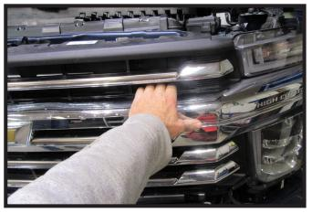
8. Grab the grill near the top and pull firmly away from the vehicle. Unsnap remaining clip near the bottom center of the grill. Remove grill and set aside to be reinstalled later.
