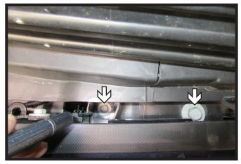
11. On the top side of the bumper, use an 18MM socket and socket extension to remove the two (2) bolts from behind the bumper. Do this on both sides of the vehicle.
