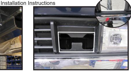
18. Trim the tow hook opening as indicated to allow room for the baseplate. Then trim the bottom inner side at an angle as needed (inset).
