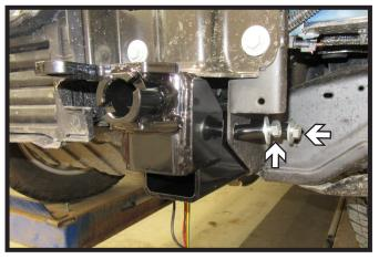
14. Slide the baseplate into the frame. Insert two (2) 1/2" bolts with lock washers, flat washers, and spacers. Do this on both sides of the vehicle.
