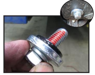
16. Insert one (1) 1/2" bolt with lock washer, thick washer, and slotted washer into the bottom of baseplate. Once bolt is started, position slotted washer and tick washer then tighten bolt. Do this on both sides of the vehicle.
