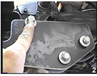
Hold the baseplate into place and insert the three
