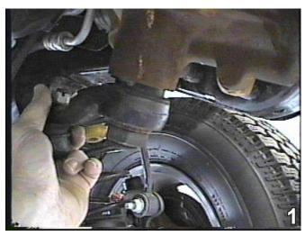
Using a 16MM socket, remove three (3) metric bolts, while having someone hold the gear box and the idler arm. Set the bolts aside to be reinstalled later.
