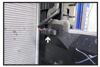
6. Remove the temperature sensor from the plastic shielding on the driver side of the vehicle. It will be repositioned later.
