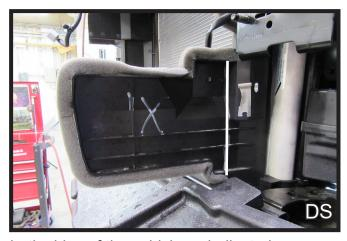
7. Using a utility knife, trim the plastic shielding on both sides of the vehicle as indicated.
