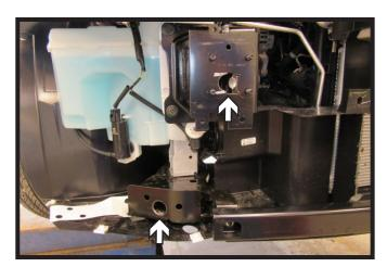
8. Using a 1-1/4" hole saw, drill two (2) access holes. Do this on both sides of the vehicle.
