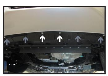
Using a 10MM socket, remove the two
