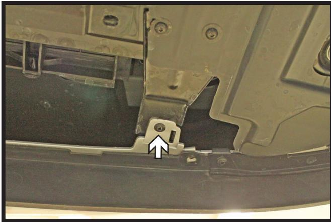
6. Using a Phillips screwdriver, remove the two (2) screws that are now visible after the removal of the belly pan. There is one (1) on each side.
