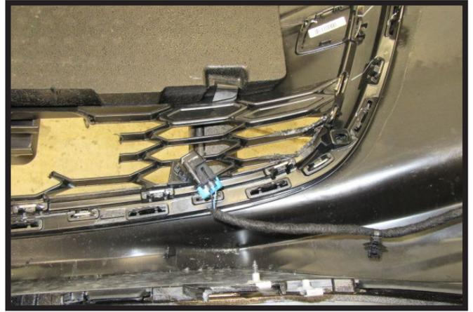
16. For vehicles with a temperature sensor, remove the sensor from the back side of the fascia on the passenger side of the vehicle. Attach sensor to the baseplate using a zip tie.
