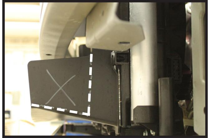
9. **Non-Turbo Vehicles:** Using a utility knife, trim the plastic shrouding as shown above. Do this on both sides of the vehicle.
