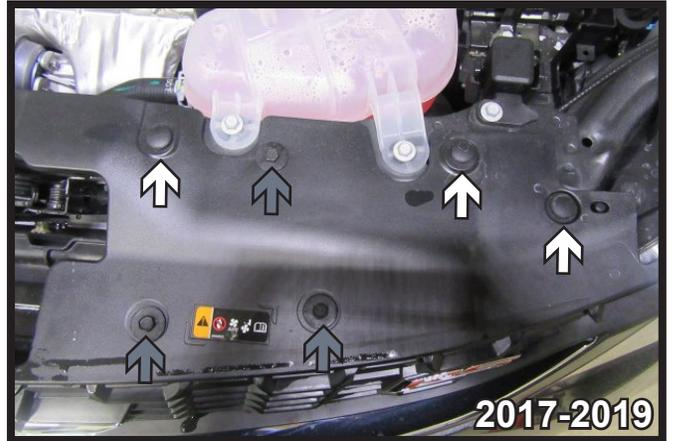
1. Remove the six (6) push pins, three (3) on each side, from the top of the plastic radiator cover (white). Using a 10MM socket, remove the four (4) bolts, two (2) on each side, from the top of the plastic radiator cover (gray).
