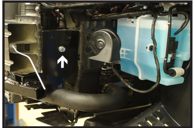
13. Slide baseplate up onto the frame of the vehicle. The baseplate support tabs on the front of the baseplate should be directly under the bumper. Be sure the baseplate is level. Clamp securely in place.
