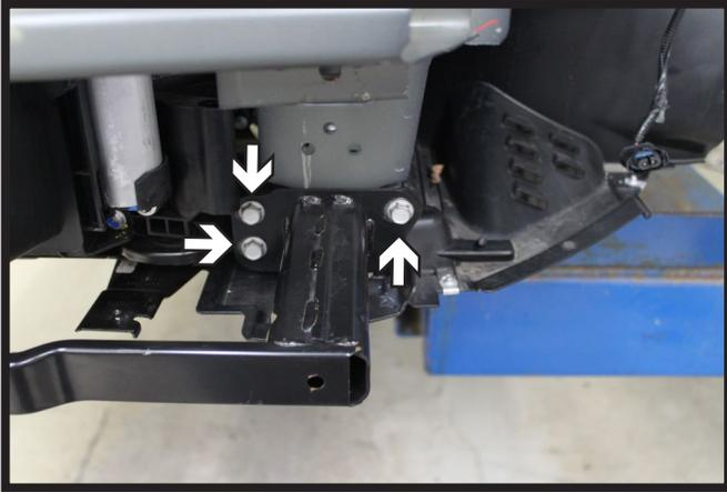
8. Using a 13MM socket, remove the three (3) bolts from the lower fascia support. Do this on both sides of the vehicle. Set the support aside.
