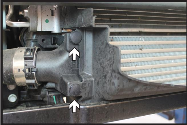
10. **RS-Models:** Remove the two (2) push pins from the plastic shroud. Do this on both sides of the vehicle. Set the shroud aside it will not be reinstalled.
