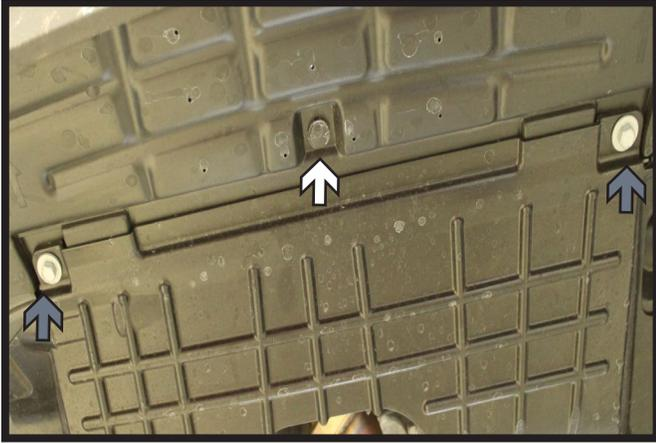
4. On the belly pan, remove the one (1) push pin (white) and with a 13MM socket, remove the two (2) bolts (gray).
