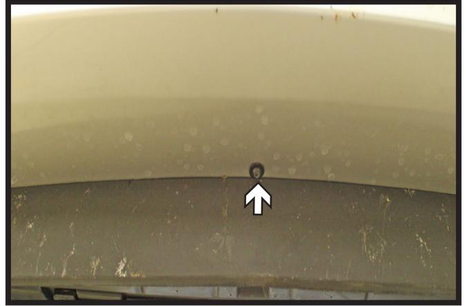
5. Underneath the license plate, with T20 Torx, remove the one (1) screw. Remove the front portion of the belly pan.
