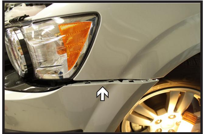
7. To remove the fascia, lift up and pull out at the fascia seam by the wheel wells. Disconnect any electrical connections and remove the fascia.
