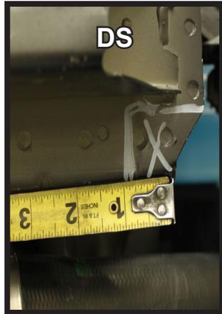
12. With a reciprocating saw, notch over 1" from the edge and upward to just slightly under the bumper. Do this on **BOTH** sides of the vehicle.
