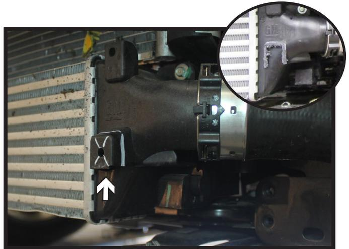
11. **RS-Models:** Trim off the lower plastic shrouding mount as shown above for baseplate clearance. Do this on both sides of the vehicle. After view is shown in inset.
