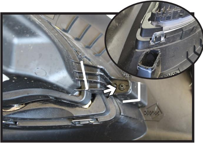
16. **RS Models:** Remove the screw on the lower fog light housing bracket. Trim off the bracket from the fog light housing and the lower mounting surface for baseplate clearance. Do this on both sides of the vehicle.
