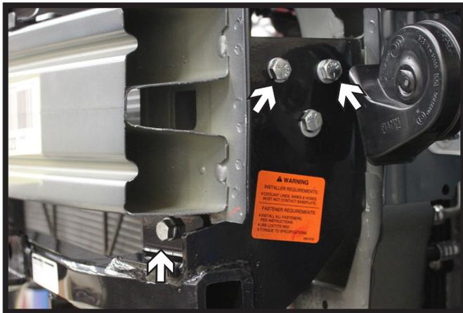
14. Drill the remaining two (2) holes at the top of the side plates and the front hole thru the frame. Install the 3/8" hardware and fully tighten all fasteners. Do this on **BOTH** sides of the vehicle.
