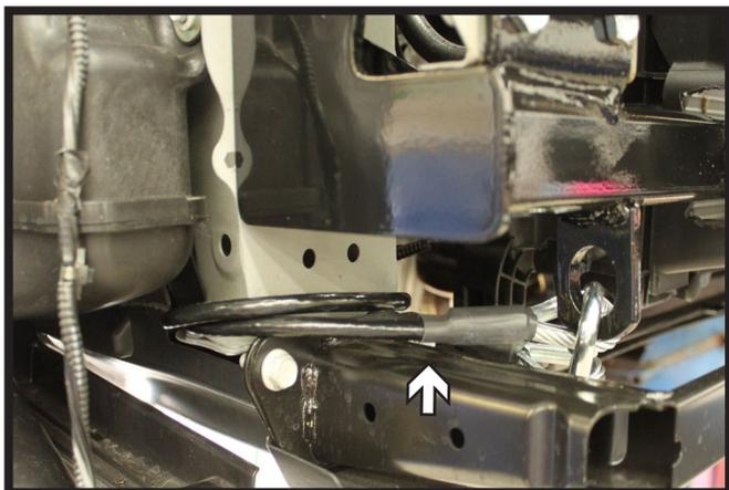
15. Attach the permanent baseplate safety cables to the provided convenience link on the baseplate. The photo above shows the recommended installation of the cables to frame of vehicle. Additional options may interfere with suggested mounting; in this case, secure the cables to a solid piece of the frame as described in the General Instructions. Be sure the safety cables do not rub against any hoses or moving parts. Do this on **BOTH** sides of the vehicle.
