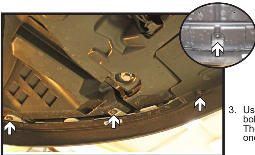
3. Using a T20 Torx, remove the seven (7) bolts from the underside of the fascia. There are three (3) on each side and one (1) in the middle (inset)
