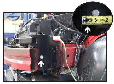
Position the baseplate onto the frame, flushing the bottom of the baseplate and frame. Leave a 1/2" gap from the front of the baseplate and the backside of the bumper (inset). Level and clamp into position.
