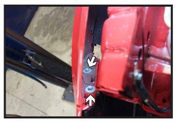
Using a 8MM socket, remove the two
