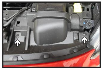
1. Remove the four (4) Phillips head push pins from the top edge of the fascia. There are two (2) on each side.
