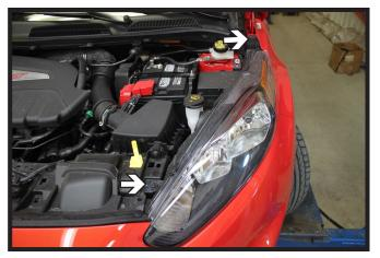
Using a T30 Torx, remove the two (2) screws from the headlight. Disconnect the electrical line and set the head light aside. Do this on both sides of the vehicle.
