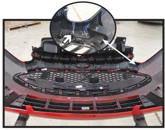
On the backside of the fascia, trim off the inner layer of the fascia along the outer groove as shown for baseplate clearance. Do this on both sides of the fascia.
