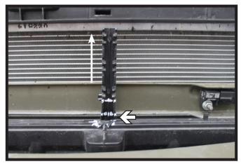
13. SFE Models: Pull up on the shutter rod. Trim off the rod flush with the base for baseplate clearance.
