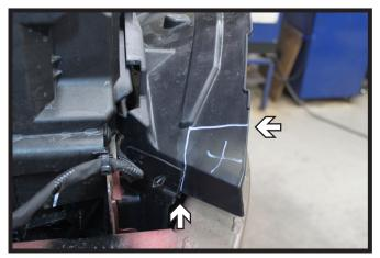
9. **ST/SE Models:** Trim the upper shrouding as shown for baseplate clearance. Do this on both sides of the vehicle.
