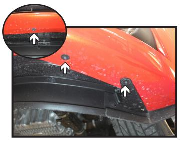
Using a 7MM socket, remove the five (5) screws from the underside of the fascia. There are two (2) in each corner and one (1) in the middle.
