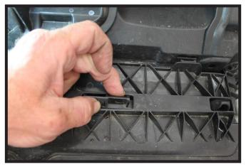
11. **SFE Models:** On top of the shutter shrouding, unsnap the two (2) clips and remove the front section of the shrouding.
