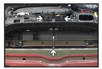
Using a 10MM socket, remove the three
