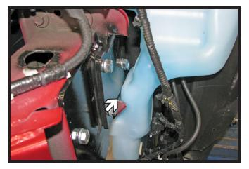
20. Reinstall the washer reservoir. Checking the clearance on the lower part of the reservoir making sure it is not rubbing on the baseplate. It should have minimum 1/16" clearance. If necessary pull the reservoir back and re-tighten the bolts.
