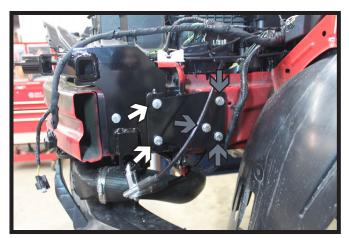
Using a 13/32" drill bit, drill the back baseplate holes thru the frame. Bolt the support bracket to the baseplate/frame with 3/8"-16 x 2" bolts, 3/8" lock washers and 3/8" nut plates (white).
