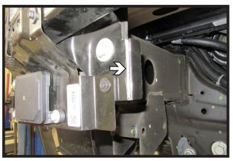
9a. **Models With ACC**: Using a saw, remove the side flange from Adaptive Cruise Control (ACC) mounting bracket.
