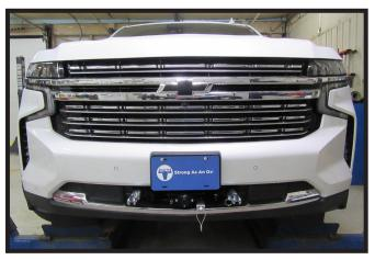
17. Hold the fascia as close to its original position as possible. Mark and trim the fascia as needed for clearance with the baseplate components. Reinstall the fascia and fascia covers.
