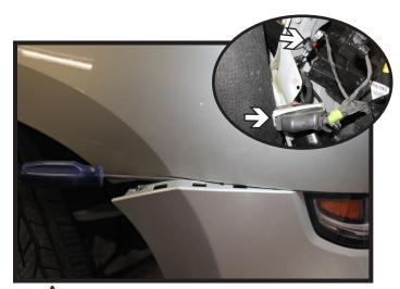
7. Gently pry the fascia loose from the front end. Carefully unplug two (2) electrical connections on the passenger side behind the facia (inset). Remove the fascia from the vehicle and set aside.
