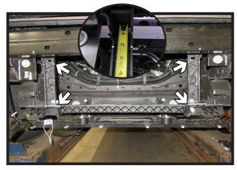
10. Using a saw, cut the two (2) vertical supports of the mounting bracket for the belly pan approximately 2" from the top and flush with the top of the lower cross member. Remove the cutout pieces.
