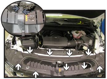
1. Remove the nine (9) push pins (white) from the fascia cover. Using a T15 Torx, remove the two (2) screws from the hood latch handle (inset gray). Set aside the facia cover and hood latch handle to be re-installed later.
