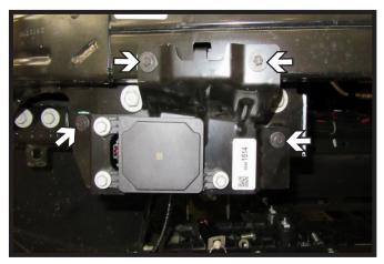
9b. **Models With ACC**: Using a 7MM socket, remove the four (4) mounting bolts from the ACC and allow to hang out of the way. This will be re-installed later.
