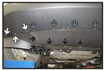
5. Using a 7MM socket, remove the three (3) bolts from the lower belly pan side cover (white). Do this on both sides. Using a T15 Torx, remove the eight (8) screws from belly pan (gray). Four (4) on each side. Using 7MM socket, remove twelve (12) bolts from belly pan (black), six (6) on each side. Remove belly pan and side covers and set aside to be re-installed later.
