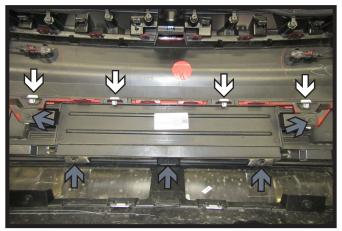
8b. **GMC Yukon**: Remove four (4) white clips from cover behind facia (white). Using a 7MM socket, remove five (5) bolts from the rear cover (gray). Remove cover and set aside. This will not be re-installed.
