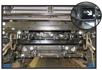
11. Slide baseplate into place. Using one (1) supplied 1/2" bolt on each side, insert into an existing hole to locate baseplate and hold in place. Using a vise grip, clamp baseplate firmly against bottom of frame on both sides.
