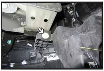
6. Using a 10MM socket, remove the one (1) bolt. Do this on both sides of the vehicle.
