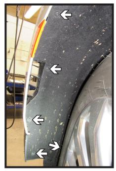
3. Using a T15 Torx, remove the five (5) screws from the wheel well liner. Do this on both sides of the vehicle.
