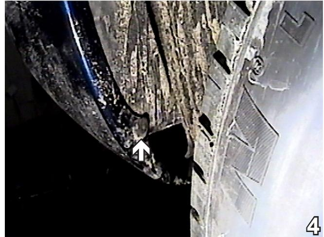
4. Just forward of the front tire, are two plastic rivets to remove using the diagonal cutters. These rivets will be replaced later with new (see the parts list).
