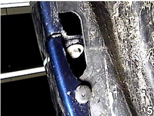
5. Using the 10MM socket, remove one metric bolt from the fascia's corner inside the wheel well. Set the bolt aside to be reinstalled later. Do this to both sides of the vehicle. Pull the fascia forward and set aside to be reinstalled later.
