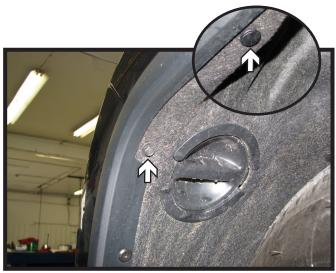
Along the upper edge of the wheel well, using a 10MM socket, remove the screw. Then remove the push pin further up (inset). Do this on both sides of the vehicle.
