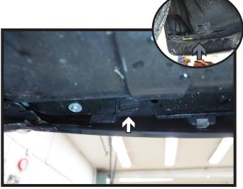
4. On the underside of the fascia, release the fascia clips by turning 90°. There is one (1) towards the middle (white) and one (1) towards the outer edge by the tire (gray). Do this on both sides of the vehicle.
