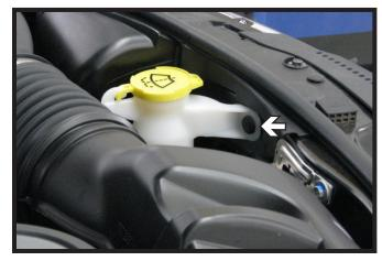
2. In the engine compartment, remove the push pin from the washer reservoir filler tube neck.
