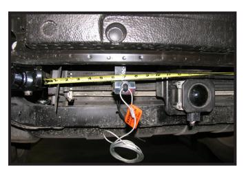
14. **Optional Breakaway:** Measure over approximately 7" from the convenience link or in the desired location, install the bracket to the bumper with a #10-16 x 1" self drilling screw. Attach the breakaway to the bracket with a 1/4"-20 x 3/4" bolt and 1/4"-20 lock nut.
