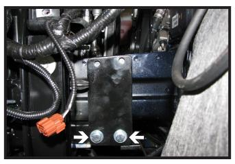
9. With the taper to the front, install the support plate onto the baseplate. Insert the 3/8"-16 x 1-1/2" bolts with 3/8" lock and flat washers into the holes and the 3/8" nut plates on the inside of the baseplate. Flush the top of the plate with the frame and tighten all hardware. Do this on both sides of the vehicle
