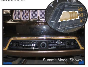
16. Hold the fascia as close to its original position as possible, mark and trim the fascia around the convenience links and attachment tabs. Reinstall the fascia. Using the plastic pop rivet gun, replace the two (2) rivets in the wheel well. Do this on both sides of the vehicle.
