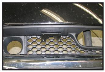
15. Install the electrical bracket to the fascia at the desired location and bent to the desired angle. With a 1/4" drill bit drill out the two (2) mounting holes thru the fascia and attach the bracket to the fascia with 1/4"-20 x 3/4" bolts and 1/4"-20 lock nuts.
