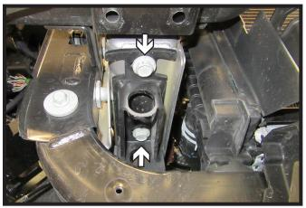
6. **Models equipped with tow hooks:** Using a 16MM socket, remove the two (2) bolts from the tow hook bracket. Remove the tow hook bracket from the vehicle. Do this on both sides of the vehicle.
