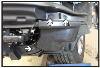
If equipped on your model of vehicle, the lower plastic shielding will need to be removed. Using a 10MM socket, remove the three (3) bolts from the shielding. Do this on both sides of the vehicle.
