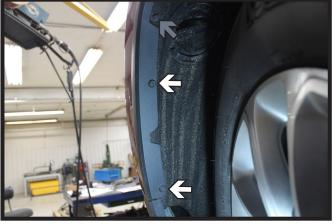
Using a utility knife, remove the two (2) plastic rivets from outer edge of the wheel well (white). Then using a 10MM socket, remove the upper screw (gray). Do this on both sides of the vehicle.
