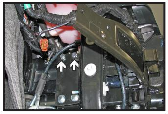
10. Using a 3/8" drill bit, drill the top two (2) holes of the support plate thru the frame. Install 3/8"-16 x 1-1/4" bolts with 3/8" lock washers and 3/8"-16 lock nuts. Do this on both sides of the vehicle. Fully tighten all hardware.
