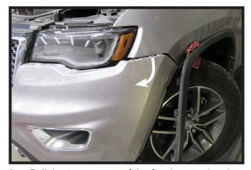
Pull the top corners of the fascia out releasing the clips behind. Continue working inward towards the grille releasing the clips under the headlights. Set the fascia aside.
