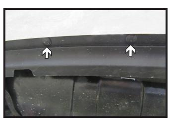
3. Underneath the bumper, remove the two (2) push pins. Do this on both sides of the vehicle.
