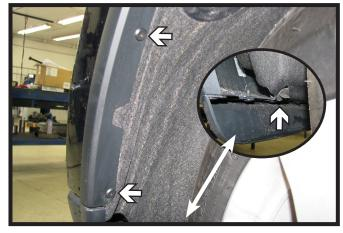
Using a utility knife, remove the two (2) plastic rivets from outer edge of the wheel well. Then release the knob at the bottom inner edge of the wheel well, by turning 90°. Do this on both sides of the vehicle.
