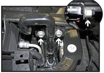
5. **Models equipped with tow hooks:** Using a 16MM socket, remove the two (2) bolts from the front side. Then using a 30MM socket or wrench, remove the nut from the backside of the tow hook. Remove the tow hook from the vehicle. Do this on both sides of the vehicle.
