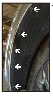
3. Using a T20 Torx, remove the five (5) screws from the outer edge of the wheel well.
