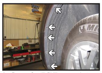
Remove five (5) Phillips screws just forward of the front tire, on the edge of fascia with a Phillips screwdriver. Do this to both sides of the vehicle. Set push pins aside to be reinstalled later.
