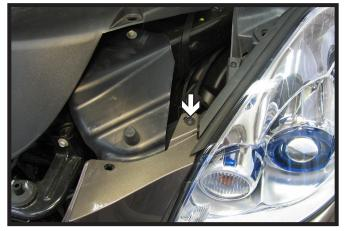
2. Using a Phillips screwdriver, remove a screw connecting the fascia near the headlight. Do this to both sides and set aside bolts for reinstallation later.
