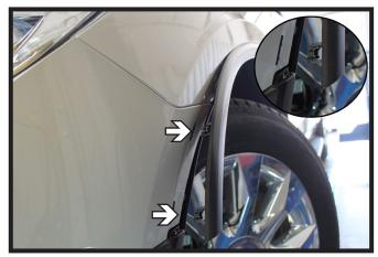
4. On 2012 models only: Once the previous step has been completed, gently pull the wheel well liner back and unclip the two (2) clips to loosen the outer trim.
