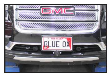
Hold the fascia as close to its original position, mark and trim the fascia around the convenience links and attachment tabs. Reinstall the fascia and fascia cover.
