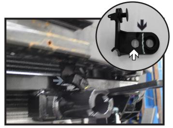
8. Hold the temperature sensor back to its original position and mark for trimming (black). Using a 7/16" drill bit, drill a new hole into the bracket on the other side of the trim line (white). Trim off the excess bracket, reinstall to the vehicle and reinstall the sensor to the bracket (gray).
