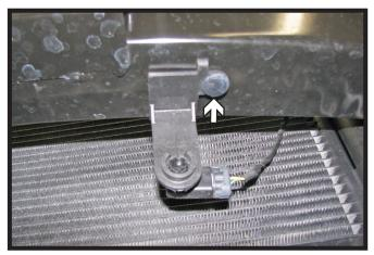
Remove the temperature sensor from the bracket, then remove the push pin from the bracket and set the bracket aside.
