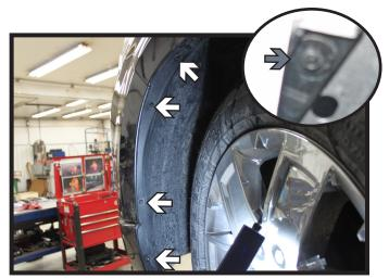
Using a T20 Torx, remove the four (4) screws from the outer edge of the wheel well (white). Then behind the wheel well cover, using a 7MM socket, remove the outer screw (gray). Do this on both sides of the vehicle.
