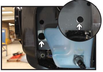
Using a 1-1/4" hole saw, drill an access hole into the frame for nut plate installation. Do this on both sides of the vehicle.
