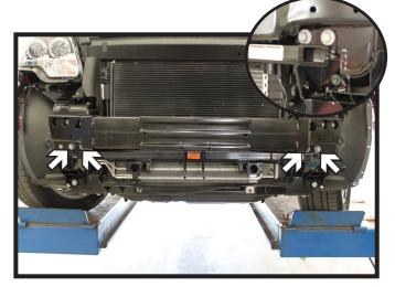
4. Using a 15MM socket, remove the four (4) bolts from the face of the bumper. There are two (2) on each side. Slide the baseplate into position, lining up the holes in the baseplate with the four (4) bumper holes. Reinstall the bolts back into the bumper and tighten.
