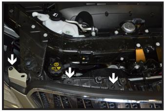
2. Along the top edge of the fascia, using a T20 Torx, remove the three (3) screws from the passenger side. Then the four (4) on the driver side.
