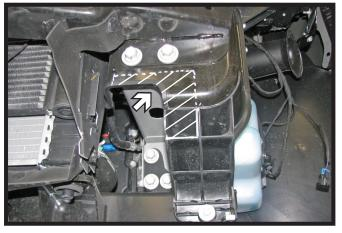
Using a reciprocating saw, notch out the shrouding for baseplate clearance. Do this on both sides of the vehicle.
