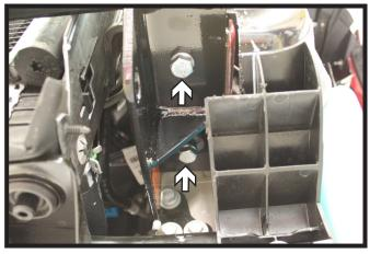
6. Using a 17/32" drill bit, drill the two (2) holes on the underside of the baseplate. Install 1/2"-13 x 1-1/2" bolts with 1/2" lock washers into the holes with 1/2"-13 nut plates inserted from the access hole. Do this on both sides of the vehicle.
