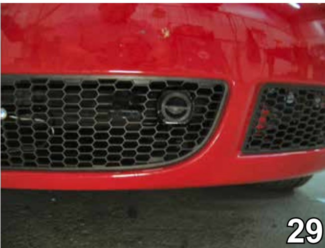
29. Reinstall the fascia and center grille, inserting all screws, pushpins, and bolts. Align the fascia to its original position and, using a diagonal cutter, trim necessary openings in the grille for attachment tabs, convenience links, and electrical rods. The installation of the baseplate is complete.
