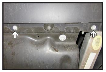
4. Using a 1/8" drill bit, drill out the one (1) rivet (gray) from the underside corner of the fascia. Using a 10MM socket, remove the two (2) bolts (white) from the underside of the fascia. Do this on both sides of the vehicle.
