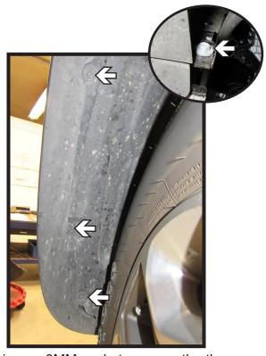
3. Using an 8MM socket, remove the three (3) bolts from the edge of the wheel well. Pull back the wheel well cover, using a 10MM socket, remove the bolt behind the trim (inset). Do this on both sides of the vehicle.
