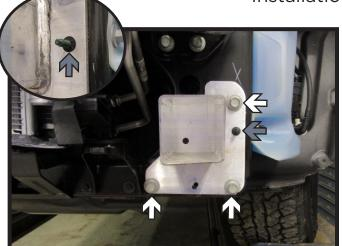
7. Using a 15MM socket, remove the three (3) bolts from the frame extension. Using a 10MM socket, remove the nut (gray) from the frame extension. Do this on both sides of the vehicle. Remove frame extension, it will not be reinstalled. Note: Some models my have a clip that needs to be removed instead of a nut (inset).
