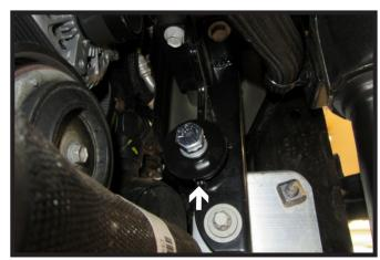
9. From the backside install the 1/2" x 5" bolt with lock washer and 1/4" x 2" DIA washer. Do this on both sides of the vehicle.
