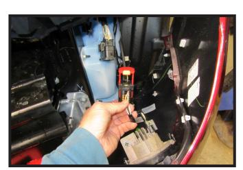
the fender and out to release. Continue along under the headlights unsnapping the fascia from the vehicle. As the fascia is removed unhook the plug on the driver side by pulling out the yellow piece and up on the red part to unhook. Remove fascia and set aside to be reinstalled later.
