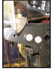
Remove the two (2) bolts from each side of the bracket near the tow hook by using an 18MM socket. Do this on both sides of the vehicle.
