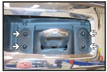
Using a 18MM socket remove the four (4) bolts indicated on both sides of the vehicle.
