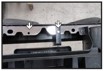
13. On the backside of the fascia there are two (2) exciting holes Use either hole to attach the electrical bracket for the tail light wiring kit using the appropriate hardware.
