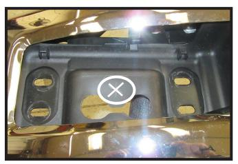
Using a utility knife remove the marked area on both sides of the vehicle to allow the baseplate to fit through the hole in the fascia.
