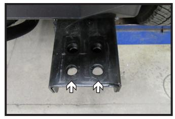
Before installing the baseplate use a 11/16" drill bit to drill out the front two (2) holes on the tow hook bracket on both sides of the vehicle.
