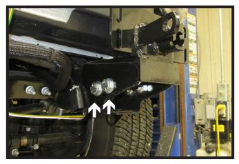
11. Use three (3) 1-3/4" bolts to attach the baseplate towards the outside of the frame. Use a flat washer on the outside and nylock nut on the inside for the front two (2) bolts indicated with a white arrows and a flat washer and nylock nut on the inside for the third bolt indicated with a gray arrow. Towards the inside of the frame use two (2) 1-3/4" bolts to attache the baseplate with the washer on the outside and nylock nut on the inside. Do this on both sides of the vehicle.
