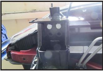
10. Slide the baseplate on, align with the existing front tow hook holes. Bolt on first using two (2) of the 5/8" x 1-3/4" bolts, and lock washers.
