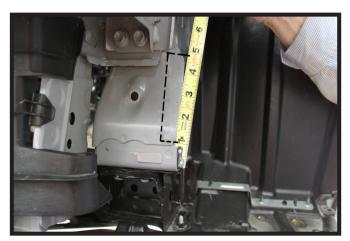
From the bottom of the frame face, measure up 1" & 4-1/2" by 3/4" deep. Using a reciprocating saw, trim a notch in the frame face. Do this to both sides of the vehicle.
