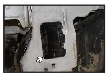
tC models only: On the driver side, remove the plastic cover along the side of the frame.
