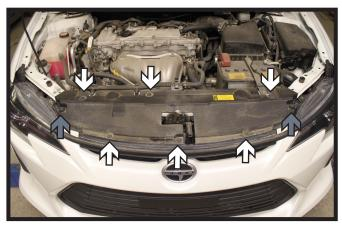
Push down on to release and remove the six (6) push pins from the fascia cover (white). Then remove the two (2) bumpers (gray) and set the cover aside.
