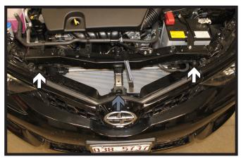
1. Remove the two (2) push pins from the fascia (white). Then, using a 10MM socket, remove the screw from the center of the fascia (gray).
