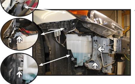
Using a 10MM socket, remove the four (4) screws from the washer reservoir (white). Remove the push pin from the reservoir neck (gray). Disconnect/plug all lines and set the reservoir aside.
