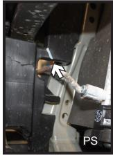
iM models only: Trim the plastic shielding under the bumper and remove the lower section.
