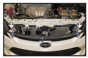
Using a 10MM socket, remove the two
