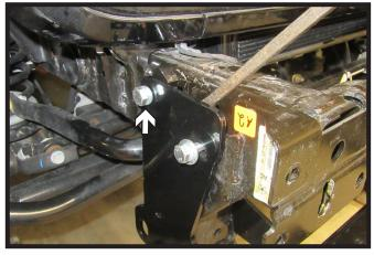
4. Loosen the top front bolt. Then insert spacer plate between the frame and the baseplate. Insert 1/2" bolt into back hole with lock washer and whiz nut. Turn the spacer plate so that it is flush with the baseplate and tighten bolt. Do this on both sides of the vehicle.
