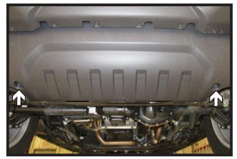
1. Using an 8MM socket, remove the two (2) bolts from the belly pan.
