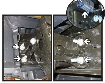
5. Using an 18MM socket, remove the four (4) nuts holding the bumper to the frame. Do this on both sides of the vehicle. On the passenger side of the vehicle unplug the indicated electrical (inset). Remove the bumper and set aside to be reinstalled later.
