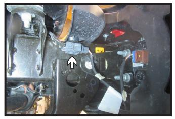
On the passenger side of the vehicle unplug the indicated electrical to allow for removal of bumper.
