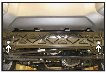
3. Using a 16MM socket, remove the two (2) bolts from the metal guard. Remove and set aside to be reinstalled later.
