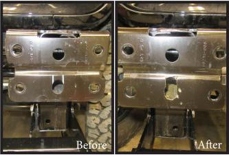
Slot the middle bottom hole on the frame as indicated and bend back to create access hole.
