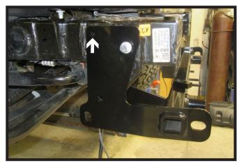
3. Using a 1/2" drill bit, drill out the top back hole on the outside of the frame using the baseplate as a template. Do this on both sides of the vehicle.
