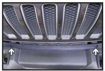
Remove the two (2) push pins, directly behind the tow hooks, from the plastic piece between the bumper and the grill. Remove and set aside to be reinstalled later.
