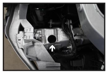
11. Disconnect the wire loom from on top of the frame. Using the existing hole as a guide, drill the hole out with the 1-1/4" hole saw bit for nut plate installation. Do this on both sides of the vehicle.
