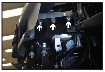
14. Align the holes in the side plate to the existing holes in the frame and loosely install the 3/8" hardware (white).
