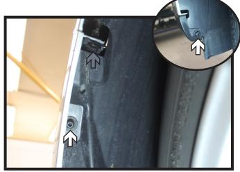
4. Using a T30 Torx, remove the two (2) screws from the edge of the wheel well (white). Also remove the push pin from the fascia/fender joint (gray). Do this on both sides of the vehicle.
