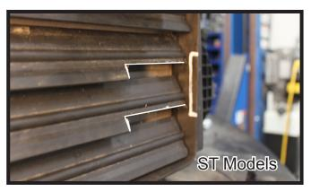
13. Hold the baseplate up to the vehicle and trim the plastic intake to allow the baseplate to be installed onto the frame.
