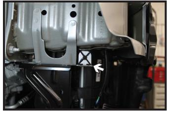
10. Trim off the washer reservoir tab on the passenger side as shown for baseplate clearance.
