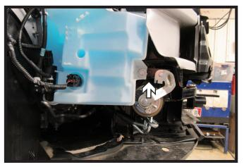
16. On the passenger side, reinstall the washer reservoir and horn using the bracket on the baseplate and the new hardware provided.
