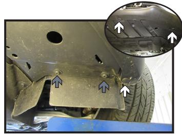
5. Remove the six (6) push pins from the underside of the fascia. There are three (3) on each side (white). Using a T30 Torx, remove the four (4) screws. There are two (2) on each side (gray).
