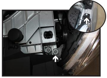
1. Using a T30 Torx, remove the two (2) screws from the headlight, disconnect and set aside. Do this on both sides of the vehicle.
