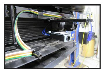
18. **Optional Breakaway:** Install the breakaway to the bracket on the baseplate with the supplied 1/4" hardware.
