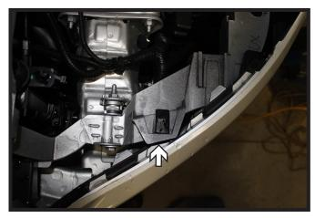
Release the clips underneath where the headlights were, pull the corners of the fascia away from the vehicle disconnecting any electrical connections and set the fascia aside.
