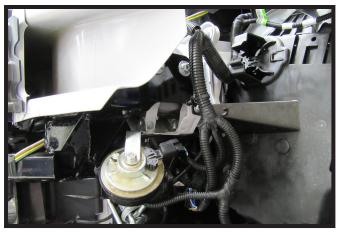
17. Bend back the webbing and reinstall the wheel well brace. Install the horn to the webbing's existing hole.
