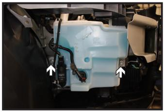
8. On the passenger side, using a 10MM socket, remove the two (2) screws from the washer reservoir. Disconnect all electrical connections. Remove and plug all fluid lines.
