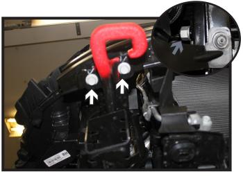
6. Using a 16MM socket, remove the two (2) bolts from the underside of the tow hook (white). Using a 30MM socket, remove the nut from the backside of the tow hook and remove from the vehicle (inset). Do this on both sides of the vehicle.
