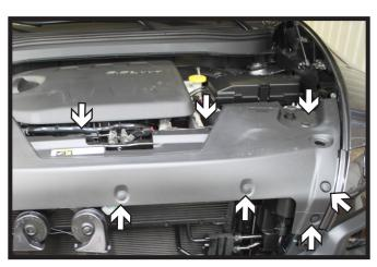
1. Remove the twelve (12) push pins from the top edge of the fascia cover and set aside.
