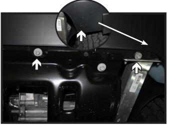
4. Remove the two (2) rivets from the underside corners of the fascia (inset). There is one (1) on each side. Using a 10MM socket, remove the four (4) screws from the middle portion of the fascia. There are two (2) on each side.
