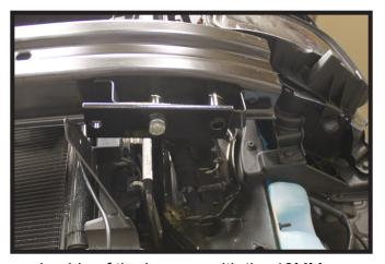
9. Loosely bolt the bumper attachment plate to the underside of the bumper with the 10MM hardware. Only install loctite onto the inner bolt (white) and fully tighten. Once the inner bolt is tightened, remove the outer bolt (gray) until the baseplate is installed. Do this on both sides of the vehicle.
