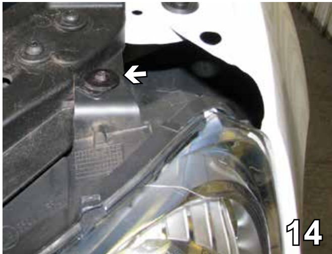
14. Use the T25 Torx to remove the bolt from the top. Do this on both sides. Pull out the headlights, disconnect and set aside to reinstall later.
