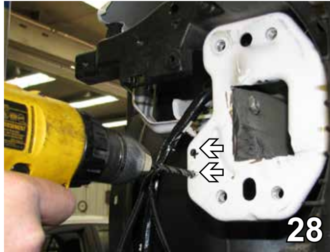
28. On the passenger side only, measure the distance between the bolts on the horn bracket, mark the frame rail end and drill with a 1/4" bit.
