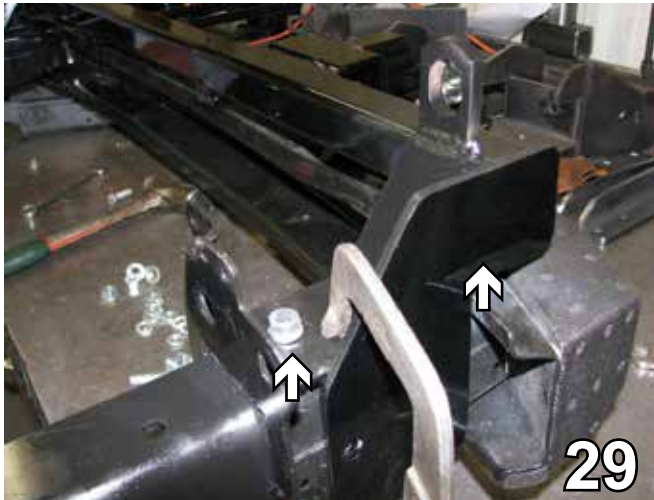
29. With the bumper upside down, slide the baseplate upside down over the outside frame extension and clamp. Align the baseplate with existing hole in the bottom of the bumper extension. Slide the driver's side frame extension bracket inside and align with the second hole back. Insert 3/8-16 x 1 1/4" bolt with 3/8" lock washer and 3/8" whiz nut. Do this on both sides.
