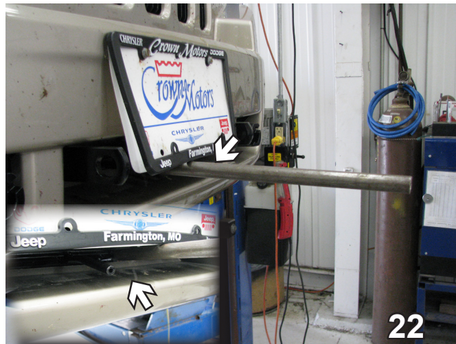
22. If the vehicle is equipped with a front license plate bracket which is in the way, insert a rod to pull it down.
