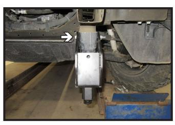
16. Slide baseplate onto tow hook housing so that the back slotted hole of the baseplate lines up with back hole on housing. Insert the one (1) 1/2" x 5" bolt as shown. Leave loose at this time. Do this on both sides of the vehicle.
