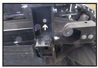
18. Using a 1/2" drill bit, drill the top rear hole on the side of the baseplate (left) and the bottom hole (right), using the baseplate as a template. Do this on both sides of the vehicle.
