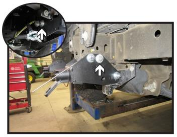
19. Install the inner front and outer back 1/2" bolts with hardware. Do this on both sides of the vehicle.
