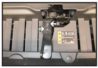
1. Using a T15 Torx, remove the two (2) bolts from the handle on the top edge of the fascia. Remove and set aside to be reinstalled later.
