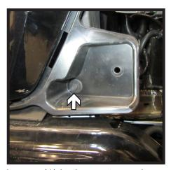
8. Using a 10MM socket, remove the three (3) bolts from the fascia, one (1) in the center and one (1) on each side.
