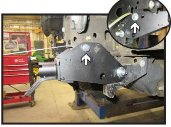
17. Rotate baseplate upward and install the outer front and inner back 1/2" bolts with hardware. Remove the back lower bolt, apply Loctite Red and reinstall. Do this on both sides of the vehicle.
