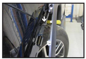
5. Unclip the fender flare and then using a 7MM socket, remove the one (1) bolt. Do this on both sides of the vehicle.
