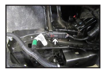
11. On the passenger side of the vehicle unplug the main wiring harness.
