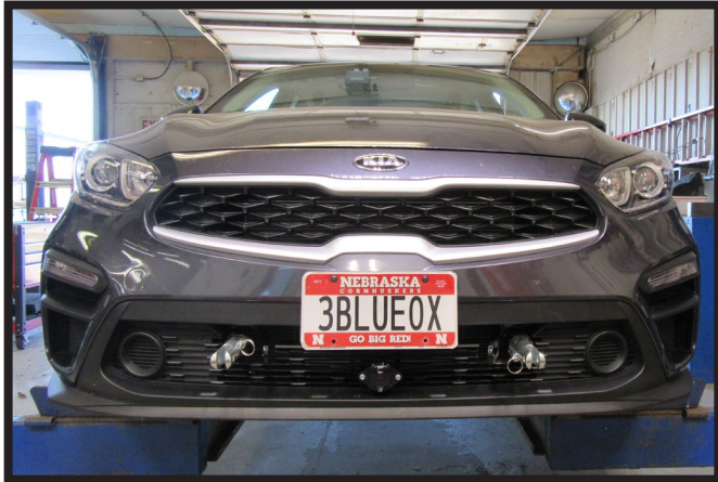
18a. 2019-2021 Models: Reinstall air baffle. Hold the fascia as close to its original position, mark and trim the fascia around the convenience links and attachment tabs. Reinstall the belly pan and fascia.
