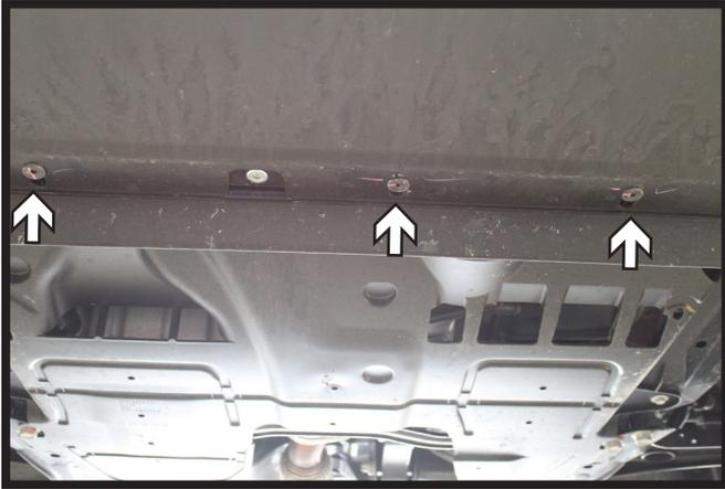
5. Using a T30 Torx, remove the three (3) screws from the bottom edge of the fascia. DO NOT remove the silver screw.
