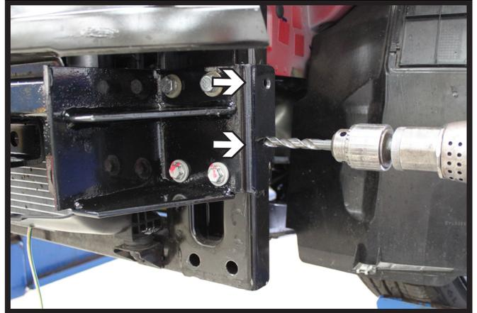
14. Using the baseplate as a template with a 13/32" drill bit, drill the two (2) side holes. Do this on both sides.
