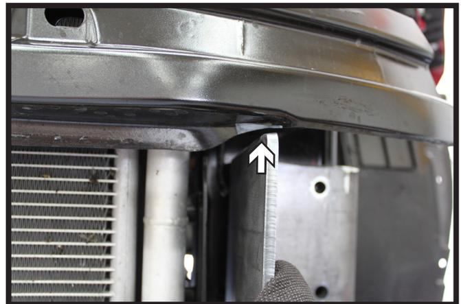
12. Hold the baseplate up to where it should slide on and mark where the frame will need to be notched to allow space. Use a reciprocating saw to make the notch. Do this on both sides.
