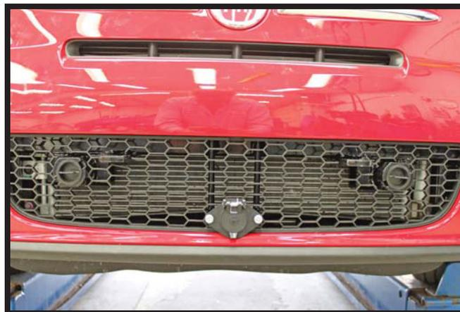
19. Align the fascia as close to its original position then mark and trim the opening for the attachment tabs and convenience links with a utility knife.
