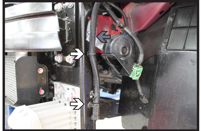
8. On the driver side, remove the two (2) clips from the frame (white). Using a 10MM socket remove the bolt from the horn bracket (gray) and unplug the wiring.
