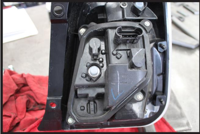
20. On the backside of the tail light, using a T20 Torx remove the four (4) screws. Remove the back piece. Do this on both sides.
