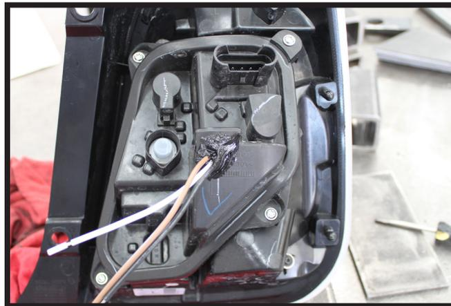
22. Using a 1/2" drill bit, drill a hole in the triangle part of the back piece. Put the wires through the hole and silicon around it. Reinstall the screws. Do this to both sides of the vehicle.
