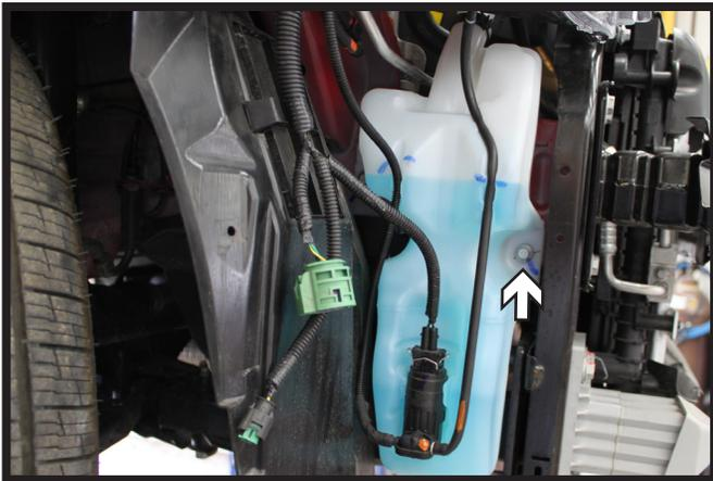
9. Using a 10MM socket, loosen the bolt on the right hand side of the washer reservoir.
