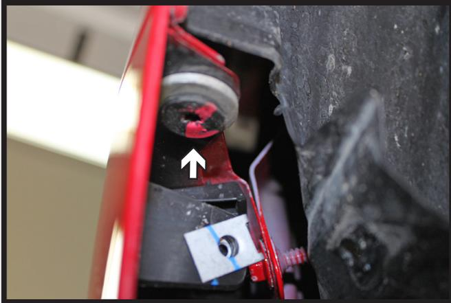
3. In the upper corner, under the wheel well cover, remove the one (1) screw with a T30 torx. Do this on both sides of the vehicle.
