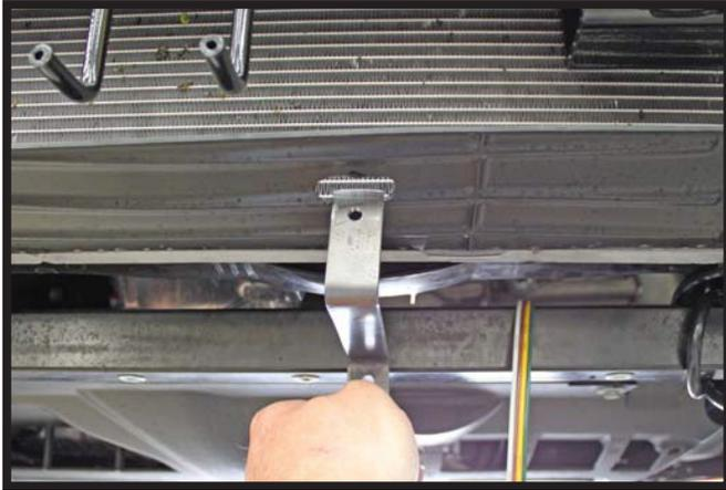
17. **Optional:** Center the breakaway bracket between the electrical rod and the convenience link and mark the plastic guard. Cut the hole for the bracket to go through with a utility knife.
