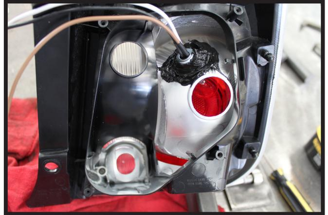
21. Using a 1/2" drill bit, drill a hole in the metal piece. Put the wires through the hole and silicon around it. Do this on both sides.
