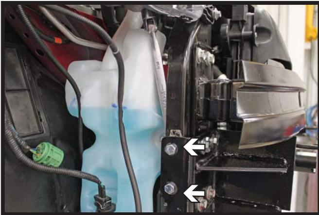
15. On the passenger side, move the windshield washer reservoir to the side. Insert 3/8"-16 x 1" bolts attach to 3/8"-16 nylock nuts. Reattach the washer reservoir. Use the same bolts and nuts on the driver side.
