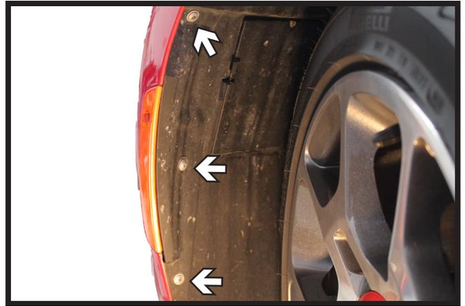
2. Using a phillips screwdriver, remove the three (3) screws from the wheel well. Do this on both sides of the vehicle.
