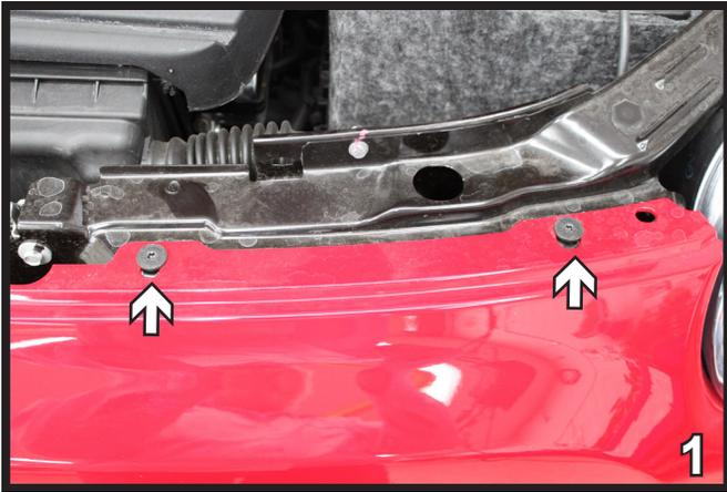
1. Using a T30 Torx, remove the four (4) screws from the top edge of the fascia. There are two (2) on each side.
