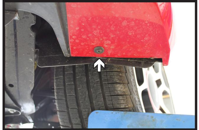
4. Using a phillips screwdriver, remove the one (1) screw from the bottom corner of the fascia. Do this on both sides of the vehicle.
