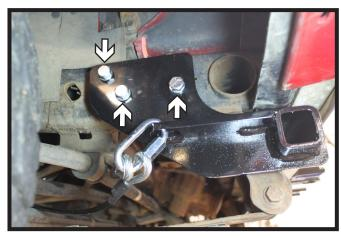
2. On the passenger side, using a 1/2" drill bit, drill the three (3) holes in the baseplate thru the frame. Install 1/2"-13 x 2-1/2" bolts with lock washers and 1/2"-13 whiz nuts on the inside of the frame. Fully tighten all hardware.
