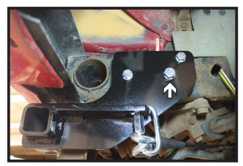
3. On the driver side, using a 1/2" drill bit, drill the middle hole in the baseplate thru the frame. Install a 1/2"-13 x 2-1/2" bolt with lock washer and 1/2"-13 whiz nut on the inside of the frame. Fully tighten the bolt.
