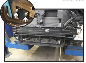
11. Pull the shielding out away from the vehicle (if applicable) and install the baseplate onto the frame with the 3/8" hardware (inset). Level the baseplate prior to fully tightening the bolts.
