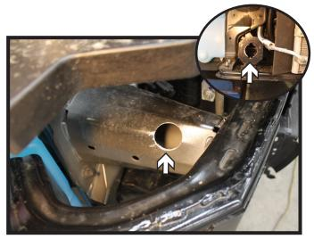
Using a 1-1/4" hole saw, drill access holes in the side of the frame as shown and in the face of the lower support (inset). Do this on both sides of the vehicle.
