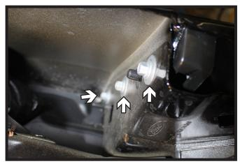
4. Using a 8MM socket, remove the three (3) screws from the fascia/fender joint underneath where the headlight was. Do this on both sides of the vehicle.
