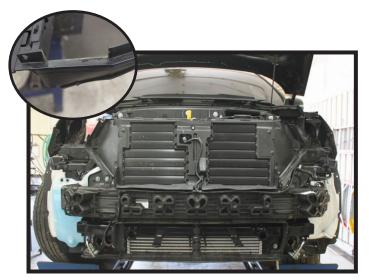
14b.**Shutter Models:** Remove the lower shutters from the shielding and trim as needed to clear the baseplate. Reinstall the shielding.
