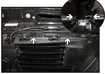
8b. **Shutter Models:** In addition to the 8a steps, using a 10MM socket, remove the four (4) screws from the top of the shielding.
