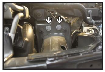
15. Along the top side of the frame, drill two (2) 3/8" holes thru both flanges, insuring enough room for the flat washers. Install the 3/8" hardware and fully tighten the bolts. Do this on both sides of the vehicle.
