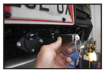
18. **Optional Breakaway:** The breakaway bracket can be installed to the license plate bracket or the lip of the fascia at the desired location with the supplied 1/4" hardware.
