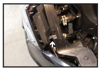
6. Unsnap the fascia by the headlight locations. Pull the corners of the fascia away from the vehicle disconnecting any electrical connections and set the fascia aside.
