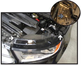
3. Using a 10MM socket, remove the two (2) screws from the headlight (white). Remove the indicated push pin from the driver side (gray). Disconnect all electrical connections and set the headlight aside. Do this on both sides of the vehicle.
