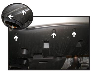
Using a 5.5MM socket, remove the ten (10) screws from the underside of the fascia. There are five (5) on each side.
