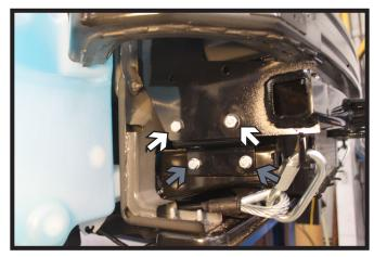
12. Install the lower support plate to the baseplate holes with the supplied 3/8" hardware (white). Then using a 3/8" drill bit, drill the lower plate holes thru the support and install the 3/8" hardware (gray). Do this on both sides of the vehicle. Fully tighten all hardware.
