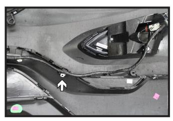
16. On the backside of the fascia, unhook the loom from the hook. Trim off the hook as necessary for clearance of the baseplate. Do this on both sides of the fascia.
