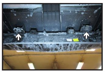
7. Using a 7MM socket, remove the two (2) bolts from the underside of the vehicle in the center.
