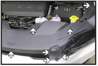
1. Remove the thirteen (13) push pins from the fascia cover. There are six (6) on each side and one (1) in the center. Remove fascia cover and set aside to be reinstalled later.
