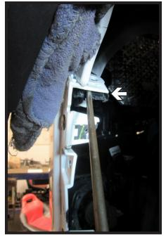
6. Unsnap the wheel well trim from the backside. Then insert a flat head screw driver between black and white pieces as shown and pull the fascia outward to remove. Do this on both sides of the vehicle.
