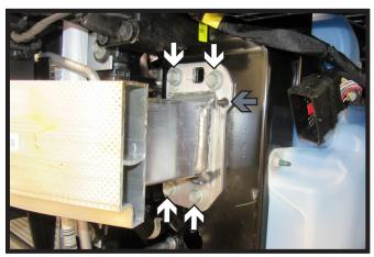
Using a 15MM socket, remove the four (4) bolts from the bumper. Using a 10MM socket, remove the nut (gray) from the bumper. Do this on both sides of the vehicle. Remove the bumper and set aside to be reinstalled later.
