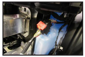
7. As the fascia is removed unhook the plug on the driver side by pulling out the yellow piece and up on the red part to unhook. Remove fascia and set aside to be reinstalled later.
