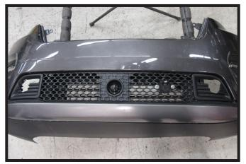
22b. **Shutter Models:** Hold the fascia as close to its original position, mark and trim the fascia around the convenience links and attachment tabs.
