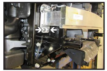
14. Install the bottom two (2) 10MM bolts with flat washers and lock washers into the bottom holes of the bumper. Do this on both sides of the vehicle.
