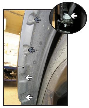
2b. **Some Vehicles:** Using an 8MM socket, remove the two (2) bolts (white) and two (2) push pins (gray) from the edge of the wheel well. Pull back the wheel well cover, using a 10MM socket, remove the bolt behind the trim (inset). Do this on both sides of the vehicle.
