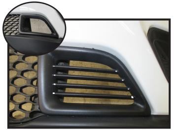
22a. **Non Shutter Models:** Remove the horizontal slats from the corner of the fascia as shown. Do this on both sides of the vehicle.
