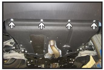
5. Using a 10MM socket, remove the four (4) bolts on the underside of the vehicle.
