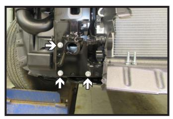
On one side of the vehicle, slide the baseplate into place and start the three (3) existing 10MM bolts with flat washers and lock washers. Snug baseplate against frame but do not fully tighten at this time.
