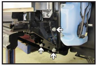
13. Slide the other baseplate onto the vehicle between the bumper and the frame. Start the three (3) existing 10MM bolts with flat washers and lock washers. Ensure the top of the baseplate is up against the bottom of the bumper on both sides of the vehicle.
