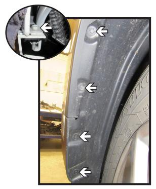
2a. **Some Vehicles:** Using an 8MM socket, remove the four (4) bolts from the edge of the wheel well. Pull back the wheel well cover, using a 10MM socket, remove the bolt behind the trim (inset). Do this on both sides of the vehicle.
