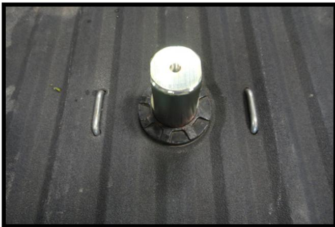
4. Install the hitch shank into the gooseneck hitch. Insure the flats of the shank are parallel to the bed ribs.
