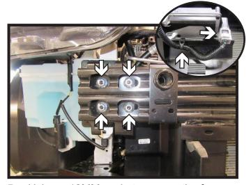
Using a 12MM socket, remove the four (4) nuts from the bumper. Do this on both sides of the vehicle. Unclip the wire loom and unplug electrical from sensor (inset).
