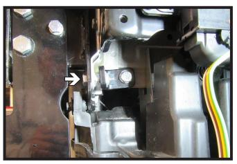
15. Insert the supplied 8MM bolt into the bottom outer hole of the frame extension. Attach hardware and angle bracket. Do this on both sides of the vehicle.
