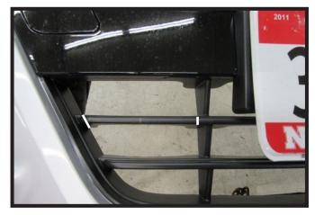
19. Using a reciprocating saw, remove the indicated piece of the fascia to allow room for the baseplate. Do this on both sides of the fascia.
