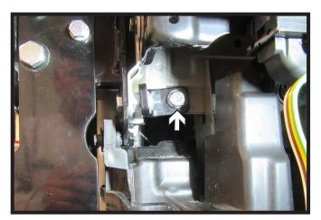
16. Using a 3/8" drill bit, drill a hole into the frame using the angle bracket as a guide. Install 3/8" bolt with hardware. Do this on both sides of the vehicle.
