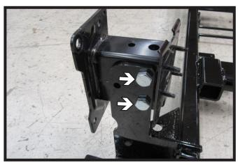
10. Using two (2) 1/2" bolts with hardware, loosely attach the horn extension to the passenger side of the baseplate.
