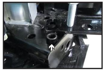
13. Place 1/2" spacer between baseplate and frame. Insert 1/2" bolt with hardware. Do this on both sides of the vehicle. Tighten all hardware at this time
