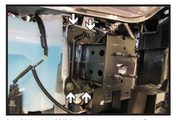
Using a 13MM socket, remove the four (4) bolts from the horn extension on the passenger side of the vehicle. Remove horn extension. It will be bolted to the baseplate before reinstallation.
