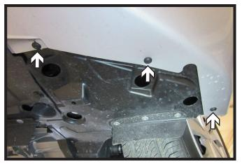
3. Using a Phillips screw driver, remove the three (3) screws from the underside of the fascia. Do this on both sides of the vehicle.
