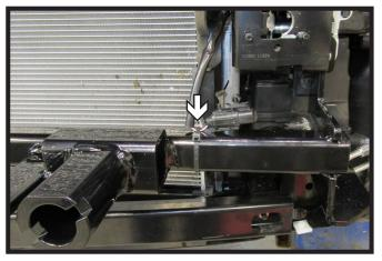
17. Attach the temperature sensor to the baseplate on the driver side of the vehicle using the supplied zip tie.
