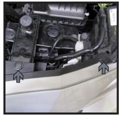
1. Using a 10MM socket, remove the two (2) bolts from the top of the fascia (white). Then remove the four (4) push pins, two (2) on each side (gray)
