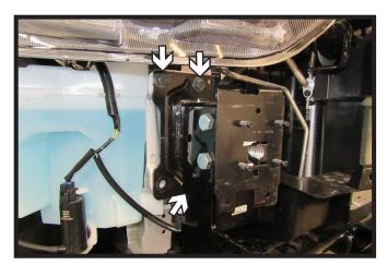
12. Reinstall the horn extension on the passenger side of the vehicle using only three (3) of the existing bolts. The bottom outer bolt on both sides of the vehicle will be installed later using supplied hardware.
