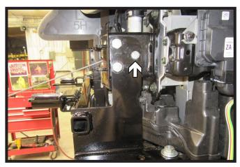
14. Using a 3/8" drill bit, drill the back hole of the baseplate. Install one (1) 3/8" bolt with hardware. Do this on both sides of the vehicle.
