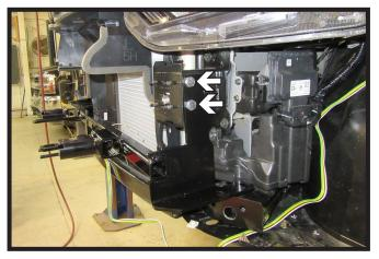
11. Slide the baseplate into place and start the front two (2) 1/2" bolts with hardware on the drive side of the vehicle.
