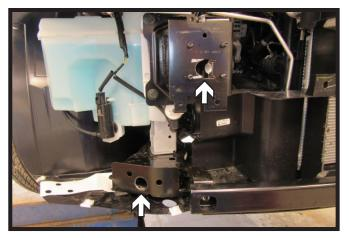
8. Using a 1-1/4" hole saw, drill two (2) access holes. Do this on both sides of the vehicle.
