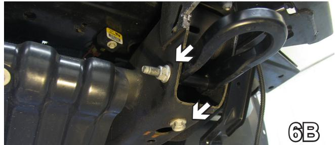
6. Using a 18MM socket, remove one bolt from the side and one bolt from the bottom of the tow hook. Do this to both sides of the vehicle. Factory tow hooks and bolts will not be reinstalled.
