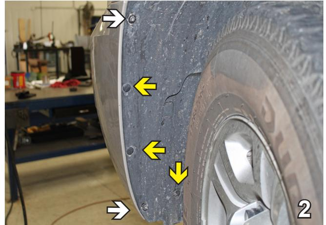
2. In front of the tire, remove two bolts with a 7MM socket (white arrows). Using a flat screwdriver, remove three push pins (yellow arrows). Do this to both sides of the vehicle. Set bolts and push pins aside to be reinstalled later.
