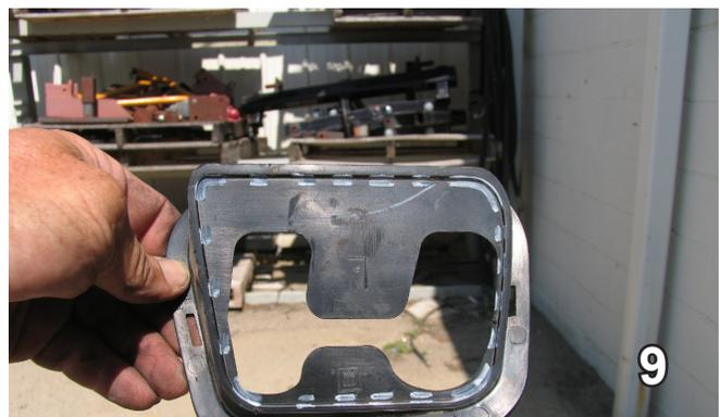
9. Using a utility knife, trim following the ridge around the backside of the guard where the tow hooks were. The photo above is what the opening should look like after your finished. Do this to both sides of the vehicle.
