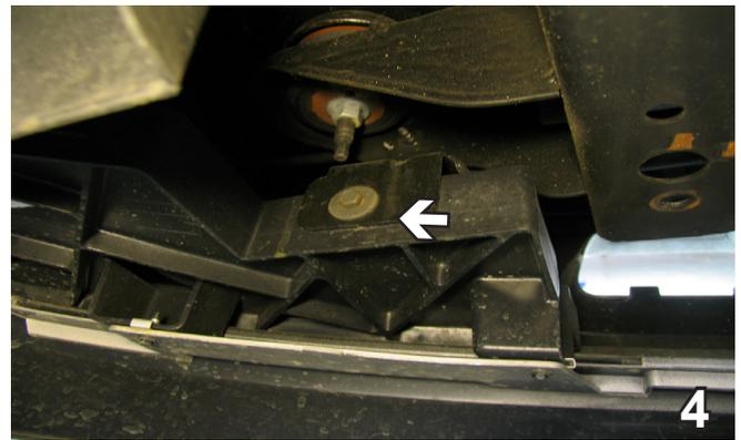
4. Using a 10MM socket, remove one bolt located underneath the fascia just left of the frame. Do this to both sides of the vehicle. Pull the fascia forward to remove. Set fascia and bolts aside to be reinstalled later.
