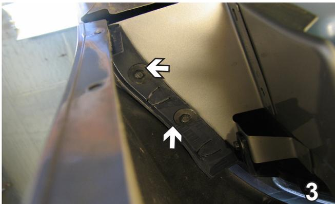
3. Using a 10MM socket, remove two bolts located just behind the wheel well plastic that we removed the bolts and push pins from. Do this to both sides of the vehicle. Set bolts aside to be reinstalled later.
