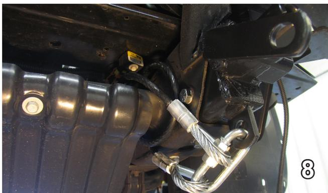
8. The photo above shows the recommended installation of the cables to frame of vehicle. If vehicle has additional options (not shown above) which interfere with mounting permanent baseplate safety cables, secure the cables to a solid piece of the vehicle frame as described in instructions included with the permanent baseplate safety cables.
