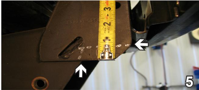
5. Using a reciprocating saw, cut along the ridge 3/4" up and straight across to remove the piece. Do this to both sides of the vehicle.
