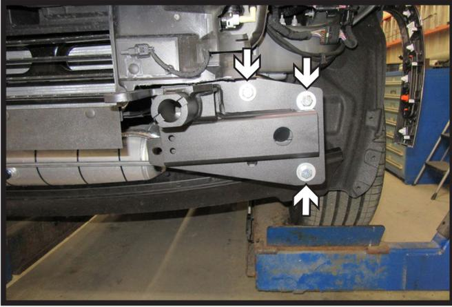
9. Hold baseplate in place and start the three (3) 1/2" x 1-1/2" bolts with flat washers and nylon lock nuts. Snug up the baseplate into place but leave loose. Do this on both sides of the vehicle.
