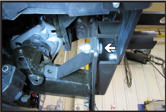
11. Attach support bracket to baseplate using one (1) 1/2" x 1-1/2" bolt with flat washer and nylon lock nut. Do this on both sides of the vehicle.
