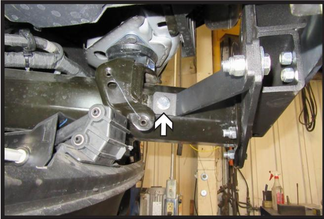
13. Install one (1) 1/2" bolt with lock washer and whiz nut. Do this on both sides of the vehicle.
