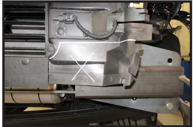
5. Remove fascia and set aside to be reinstalled later. Unplug the electrical on both sides of the vehicle as the fascia is removed.
