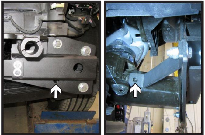
12. Using a 1/2" drill bit, drill the bottom inside hole on the front of the baseplate (left). Then using the support bracket as a template, drill 1/2" hole in frame (right). Do this on both sides of the vehicle.
