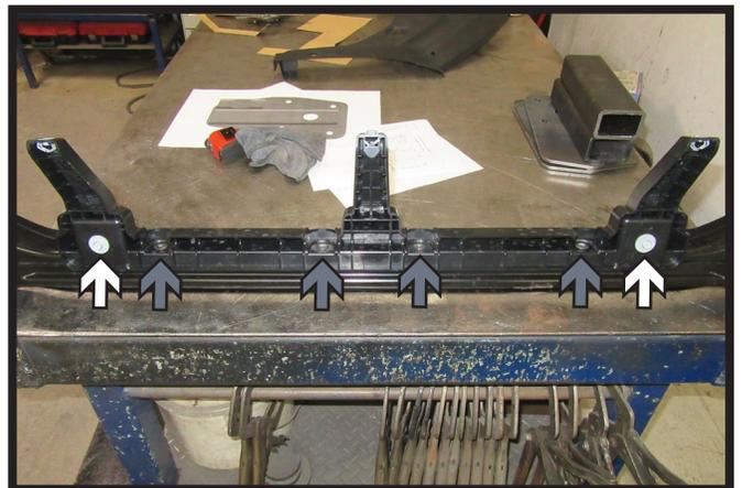
8. Using a 10MM socket, remove the two (2) bolts (white) from the plastic piece on the bottom of the bumper. Then using 1/4" drill bit, drill out the four (4) plastic rivets (gray). Remove plastic piece and set aside to be reinstalled with the baseplate.
