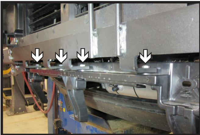
15. Attach plastic piece from bumper to cross member using four (4) 1/4" x 1" bolts with flat washers and lock washers.
