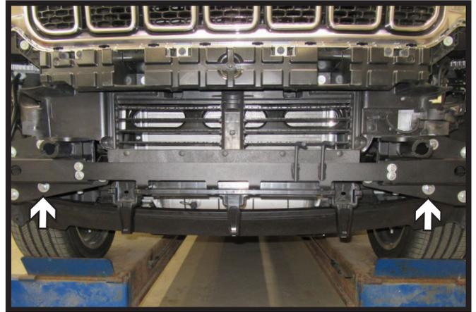
14. Install two (2) 1/2" x 1-1/2" bolts with flat washers and nylon lock nuts into the bottom inside holes on the front of the vehicle.
