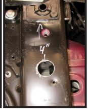
17. Measure 4" down from the bottom of the frame end and mark on the driver side of the vehicle. Using a 1-1/4" hole saw, drill an access hole centered over mark on the frame
