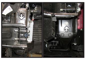
10. Using a 16MM socket, remove the two (2) bolts (white) from the bumper. Then using a 10MM socket, remove the one (1) nut (gray). Do this on both sides of the vehicle. Remove bumper and set aside. It will not be reinstalled later.
