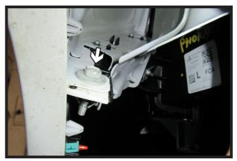
5. Pull back the wheel well liner. Using a 10MM socket, remove the one (1) bolt from the fascia joint. Do this on both sides of the vehicle.
