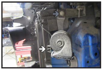
Unclip horn from the bracket (white). Then using a 10MM socket, remove the one
