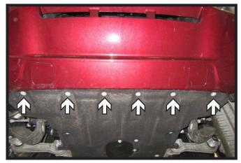
7a. **Non-Hybrid (4xe) Models**: Using a 10MM socket, remove the six (6) bolts from the belly pan.
