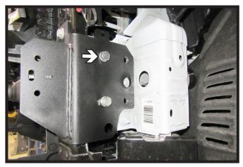
21. Insert spacer plate at top of baseplate between the frame and baseplate with the slotted end facing downward. Once spacer plate is in position insert 1/2" x 1-1/2" bolt with lock washer and whiz nut into top front hole.
