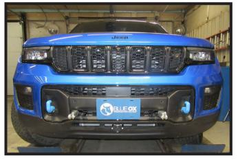
29b. **Hybrid (4xe) Models**: Hold the fascia as close to its original position, mark and trim the fascia around the convenience links and attachment tabs. Reinstall the fascia and fascia cover. Reconnect all electrical connections and hose.
