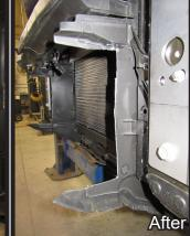
14. Using a utility knife, cut and remove the area from plastic shroud as shown. Do this on both sides of the vehicle.
