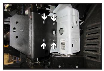
19. Using 1/2" drill bit. Drill the four (4) holes (white) on the side of the frame using the baseplate as a template. Do this on both sides of the vehicle.
