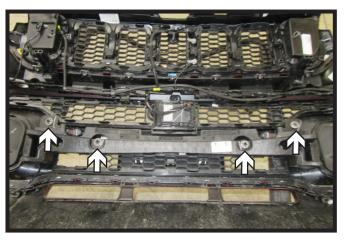
28. Remove the four (4) clips attaching the foam piece to the back of the fascia. Remove foam piece, it will not be reinstalled.
