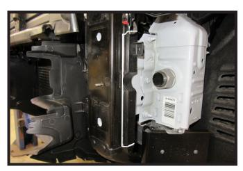
13. Using a reciprocating saw, trim the frame as indicated. Do this on both sides of the vehicle.
