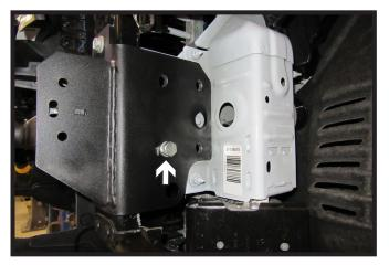
20. Start a 1/2" x 1-1/2" bolt with lock washer and whiz nut in the bottom front hole. Leave loose at this time. Do this on both sides of the vehicle.
