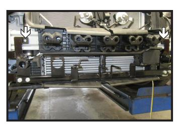
21. Using a 1/2" drill bit drill out top two (2) holes one (1) on each side. Metal is extremely hard so may need to start with a 1/4" drill bit then work up to a 3/8" drill bit and then eventually use a 1/2" drill bit to create the holes. Make sure to drill slowly.
