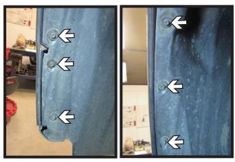
4. Using a 5.5MM socket, remove the six (6) bolts from the edge of the wheel well. Do this on both sides of the vehicle.
