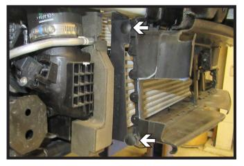
Remove the two (2) push pins and then remove the back plastic piece to allow baseplate to fit.
