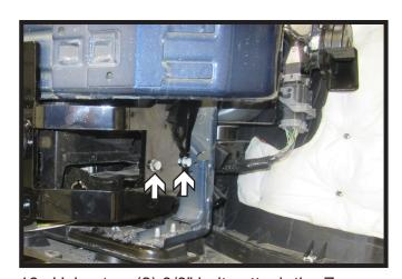
Using two (2) 3/8" bolts attach the Z bracket to the side plate as indicated.
