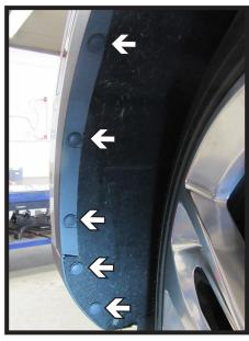
4. Remove the five (5) push pins from along the edge of the wheel well. Do this on both sides of the vehicle.
