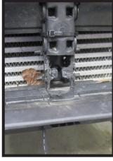
11. Trim the shutter housing on both sides of the vehicle and in the middle as shown to allow room for the baseplate cross member.
