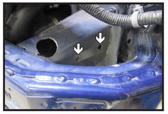
14. Using a 3/8" drill bit, ream out the rear existing hole. Do this on both sides of the vehicle.
