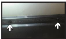
6. Using a 5.5MM socket, remove the eighteen (18) screws from the underside of the fascia. There are eight (8) on each side and two (2) in the center.
