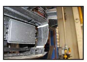
8a. Using a reciprocating saw, trim out the section of shielding as shown.
