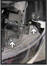
Using a T25 Torx, remove the four (4) screws from above the headlights. There are two (2) on each side.
