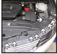
1. Remove the five (19) push pins from along the edge of the fascia. There are eight (8) on each side and three (3) in top middle. Remove top cover.
