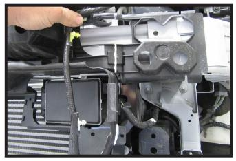
On the driver side of the vehicle remove the wiring harness from the push pin bracket. Using a utility knife remove the indicated areas
