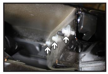
Using a 8MM socket, remove the three
