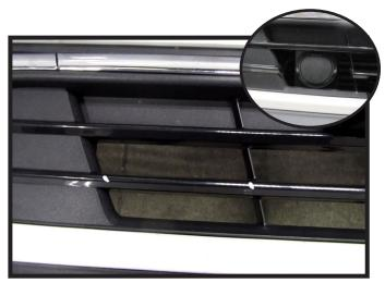
25. Optional: If there is an electrical plug for the engine block heater on the passenger side of the vehicle the following piece will need to be removed from the grill area as indicated.
