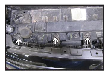
2. Using a 10MM socket, remove the six (6) bolts from the top of the fascia. There are three (3) on each side.
