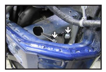
15. Hold up the side bracket and start the top two (2) 3/8" bolts. Use a lock washer with the front bolt. For the back bolt use a flat washer and a lock washer. Make sure the bracket is level and tighten. Do this on both sides of the vehicle.
