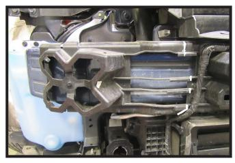
12. Using a reciprocating saw, cut the corner plastic piece off of the driver and passenger side where marked and remove plastic piece.
