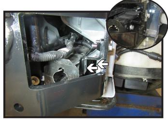
20. Before attaching the safety cables drill out bottom two (2) indicated holes using a 3/8" drill bit. Then insert two (2) 3/8" bolts with lock washers. Do this on both sides of the vehicle.
