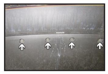
6. Using a 5.5MM socket, remove the ten (10) bolts from the underside of the fascia. There are three (3) on each side and four (4) in the middle. Pull the corners of the fascia away from the vehicle disconnecting any electrical connections and set the fascia aside to be reinstalled later.
