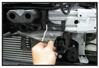
12. Using a utility knife remove the indicated area above the adaptive cruise control sensor on the driver side of the vehicle.
