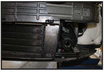
7b. **Shutter Models without ACC Only:**Remove the shield on the driver side next to the shutter support.
