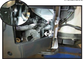
23. Before attaching the safety cables drill out bottom two (2) indicated holes using a 3/8" drill bit. Then insert two (2) 3/8" bolts with lock washers. Do this on both sides of the vehicle.
