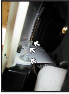
5. Pull the wheel well liner back and remove the three (3) bolts using a 8MM socket. Do this for both sides of the vehicle.
