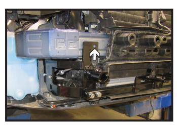
19. Insert one (1) 1/2" bolt with spacer on the back side. If the spacer cannot be attached perfectly up and down, may need to angle spacer slightly to get it to fit. Do this on both sides of the vehicle.
