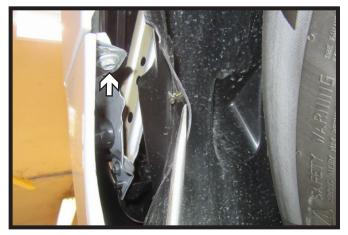
2. Using a flat head screw driver, pull back the wheel well liner. Then using a 10MM socket, remove the one (1) bolt. Do this on both sides of the vehicle.
