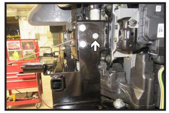
15. Using a 3/8" drill bit, drill the back hole of the baseplate. Install one (1) 3/8" bolt with hardware. Do this on both sides of the vehicle.
