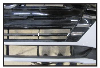
20b. **2023 Models**: Using a reciprocating saw, remove the indicated piece of the fascia to allow room for the baseplate. Do this on both sides of the fascia.
