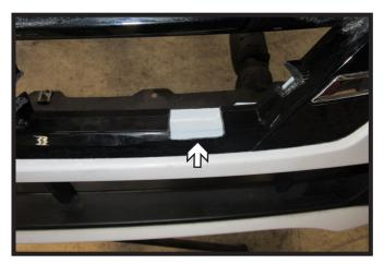
21. **2023 Models**: The bottom black piece on fascia may need to be notched for baseplate clearance. Hold the fascia as close to its original position, mark and trim the fascia around the attachment tabs.
