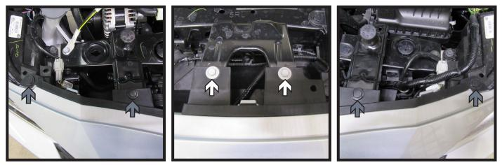
1. Using a 10MM socket, remove the two (2) bolts from the top of the fascia (white). Then remove the four (4) push pins, two (2) on each side (gray)
