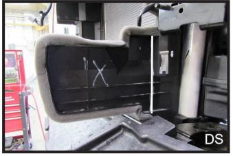
8. Using a utility knife, trim the plastic shielding on both sides of the vehicle as indicated.
