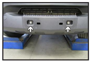
6. Using a 13MM socket, remove the two (2) screws from the front of the fascia.
