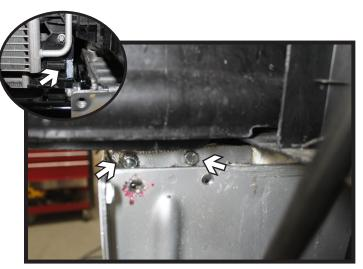
13. Using a 3/8" drill bit, drill thru the frame lips into the top baseplate holes. Install the 3/8" hardware into the top holes and fully tighten. Do this on both sides of the vehicle. Note: the plastic shielding behind may need to be trimmed for easier nut access (inset).
