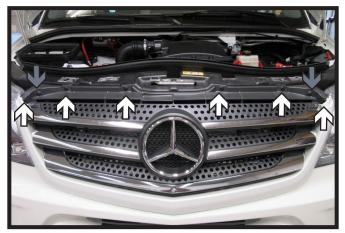
1. Remove the six (6) push pins from the top of the grille (white). Using a T25 Torx, remove the two screws (gray).
