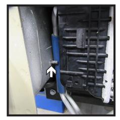
11. On the passenger side, using a 8MM socket, remove the bolt from the compressor line bracket (left). Pull the lines forward, then using a 10MM wrench, remove the nut from the bracket (middle). Set the bracket aside it will not be reinstalled.
