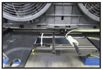
15. Install the wire loom cover around the condensor lines to prevent rubbing (left). And zip-tie the line to the baseplate to prevent it from moving around (right).
