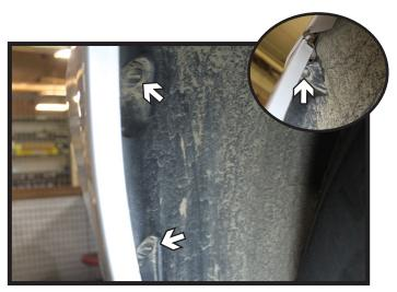
2. Remove the three (3) push pins in the wheel well. Do this on both sides of the vehicle.
