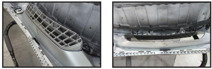
16. On the back side of the fascia, trim off the inner grille at the joint all the way around.
