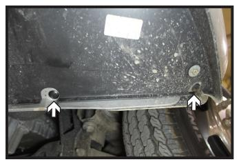
3. Remove the four (4) push pins from the underside of the fascia. There are two (2) on each side.
