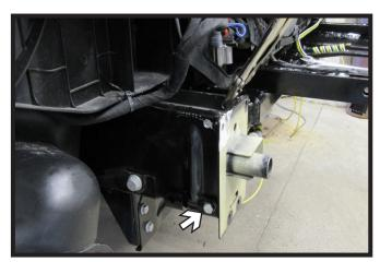
12. Clamp the baseplate to the frame of the vehicle. Using a 3/8" drill bit, drill the lower front baseplate hole thru the frame. Install the 3/8" hardware into the hole and fully tighten. Do this on both sides of the vehicle.
