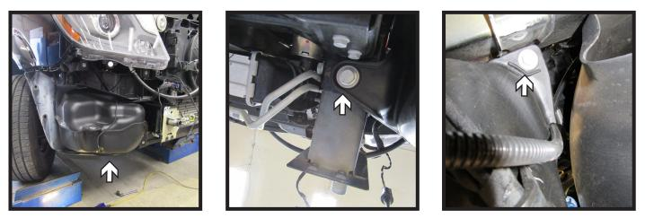
10. On the passenger side, using a 18MM socket, remove the front bolt (middle) from the tank. Then using a 13MM socket, remove the rear bolt (right) and let the tank hang down.
