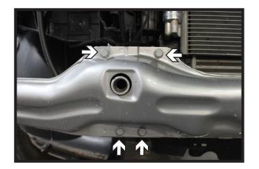
9. Using a 13MM socket, remove the eight (8) bolts from the bumper. There are four (4) on each side.
