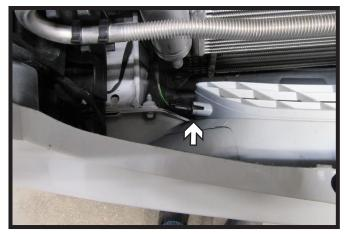
8. On the passenger side behind the fascia, remove the temperature sensor.
