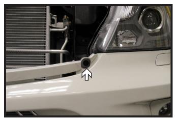
7. After removing the grill, using a T20 Torx, remove the two (2) screws from under the grill area. There is one (1) on each side.
