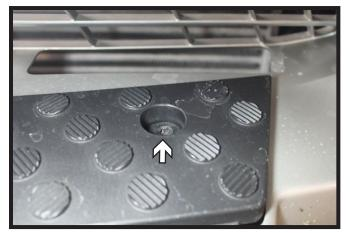
5. Using a T45 Torx, remove the two (2) screws from the step area on top of the fascia. There is one (1) on each side.
