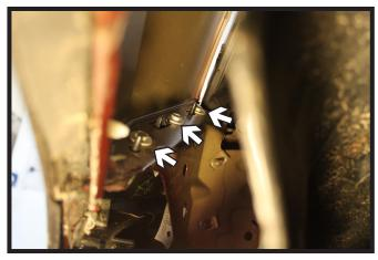
Using a 10MM socket, pull back the wheel well liner and remove the three (3) screws from the fascia joint. Do this on both sides of the vehicle.
