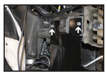
14. Using a 3/8" drill bit, drill the upper two (2) holes on the side of the baseplate thru the frame. Install the 3/8" bolts (white) as indicated and instert wire nuts through the hole in the frame (gray), fully tighten. Do this on both sides of the vehicle.
