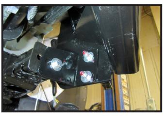
13. Install the 3/8" hardware into the existing holes and fully tighten the bolts. Do this on both sides of the vehicle.
