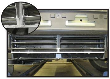
10. Using a reciprocating saw, trim the marked area to be flush with the shielding. Also, trim the middle plastic about 1-1/2" up to the bottom shutter, ensuring it is also flush with the plastic shielding.
