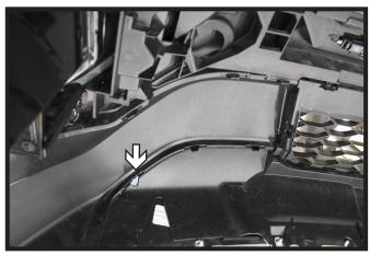
17. On the backside of the fascia trim the outer tab shown flush with the backside of the fascia for clearance of the baseplate.
