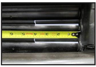
9. Using a reciprocating saw, trim the bottom two shutters, 4" across and roughly 1/2" deep. Do this for both sides of the vehicle.
