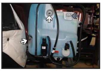
6. Using a 11MM socket, remove the two (2) nuts from the washer reservoir (white). Then using a 8MM socket, remove the screw (gray). Disconnect/plug all lines and set the reservoir aside.
