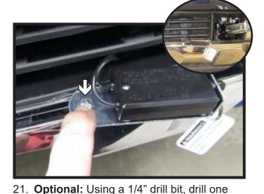
(1) hole on the driver side of the vehicle.
