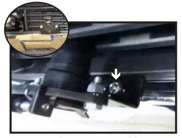
20. Using a 1/4" drill bit, drill two (2) holes on the passenger side of the vehicle using the electrical bracket as a guide. Insert two (2) 1/4" bolts with hardware. Note: Install where indicated to run electrical through opening in fascia and avoid shutters (inset).
