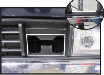
18. Trim the tow hook opening as indicated to allow room for the baseplate. Then trim the bottom inner side at an angle as needed (inset).
