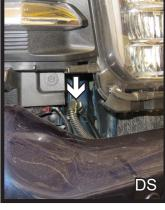
12. Disconnect the indicated wire loom on the driver side of the vehicle and the main wire loom on the passenger side of the vehicle. Remove bumper and set aside to be reinstalled later.
