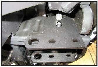
Attach inner side plate using a 1/2" bolt with lock washer and nut plate. Leave loose. Do this on both sides of the vehicle.
