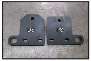
There are two (2) support brackets styles for each side of the vehicle. The tapered edge brackets are for the driver side of the vehicle and the square edge brackets are for the passenger side of the vehicle. Note: The plates with the welded spacer are installed toward the inside of the vehicle.
