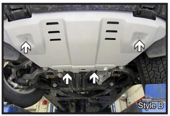
6. Using a 15MM socket, remove the front two (2) bolts of the belly pan. Loosen the back two (2) bolts then slide belly pan off and set aside to be reinstalled later.
