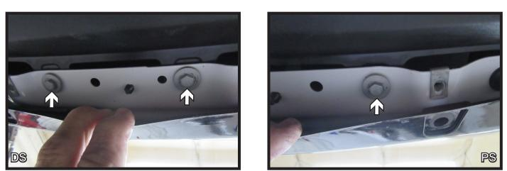
3. **For Vehicles with a Shroud:** Pull down the front of the plastic shroud. Using a 10MM socket, remove the three (3) bolts. Two (2) from the driver side and one (1) from the passenger side of the vehicle.
