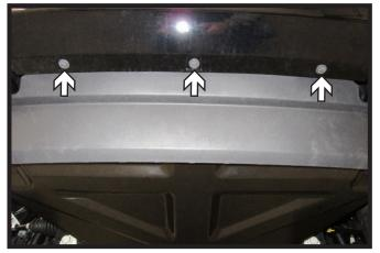
2. For Vehicles with a Shroud: Using a 10MM socket, remove the three (3) bolts from the front of the plastic shroud.
