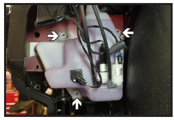
On the driver side, using a 10MM socket, remove the three (3) nuts from the washer fliud reservoir. Disconnect all lines and electrical connections, then set reservoir aside.
