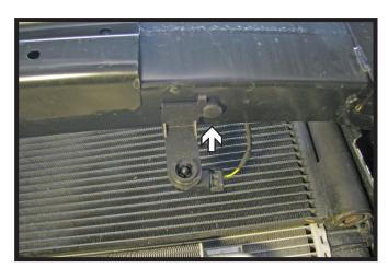
6. On the driver side, remove the push pin from the temperature sensor and temporarily move above the bumper. The sensor will be relocated later.
