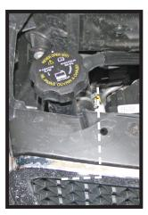
8. Using a reciprocating saw, trim an area on the frame approximately as shown. Cut the bottom flush with the bottom rail (gray) and vertically just inside the rib (approximately 1-5/8") then 2-1/2" back at the top. Do this on both sides of the vehicle.
