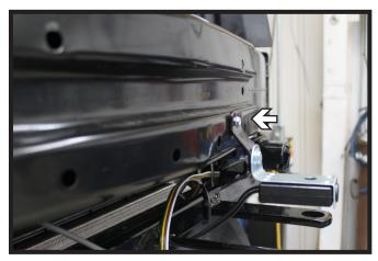
14. **Optional Breakaway:** Attach the bracket to the metal bumper with the #10-16 x 1" self drilling screw at the desired location. Attach the breakaway to the bracket with the 1/4" hardware provided.
