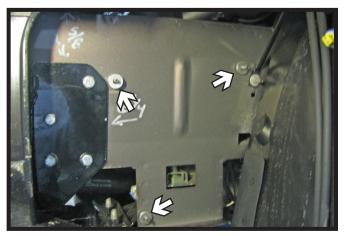
11. On the driver side, place six (6) 1/4" flat washers onto each of the washer reservoir studs. Reinstall the reservoir and horns.
