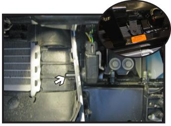
12. Reinstall the temperature sensor to its original location or on the driver's side, using a 1/2" drill bit, drill a hole into the plastic shrouding. Then snap the temperature control into the hole.
