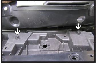
2. Lift up fascia cover. Using a 10MM socket, remove the two (2) bolts from the top of the fascia. Do this on both sides of the vehicle.
