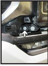
5. Using an 8MM socket, remove the two (2) inside bolts, one (1) on each side of the vehicle.
