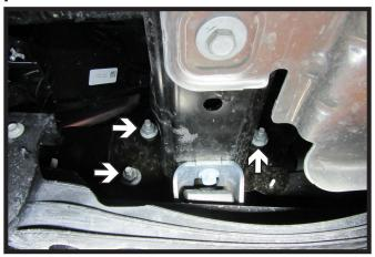
Using a 21MM socket, remove the three
