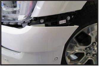
Remove the middle fascia piece by grabbing the edge and pulling outward. Set piece aside to be reinstalled later.
