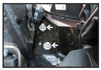
7. Coming from underneath the vehicle, use a 21MM socket to remove the two (2) outer nuts from behind the bumper. Do this on both sides of the vehicle.
