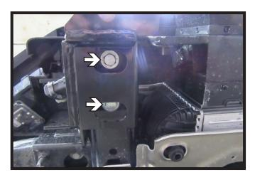
Slide baseplate onto tow hook housing and install two (2) 1/2" bolts with hardware into the bottom holes. Do this on both sides of the vehicle.
