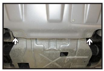
1. Using a 15MM socket, remove the two (2) bolts for the back of the belly pan.
