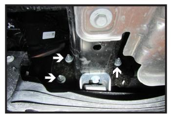
Using a 21MM socket, remove the three
