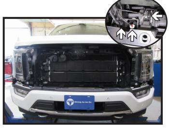
Lift the fascia cover and unplug the electrical connections (inset). Remove fascia and set aside to be reinstalled later.
