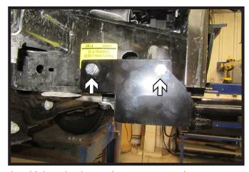
4. Using the baseplate as a template, use a 1/2" drill bit to drill two (2) holes through the frame of the vehicle. Install two (2) 1/2" bolts with hardware. Do this on both sides of the vehicle.
