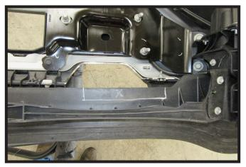
Hybrid Models: On the backside of the fascia, trim the plastic behind the tow hook opening to allow clearance for the baseplate. Do this on both sides of the vehicle.
